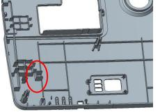
3. The parts highlighted in red were added to the bottom cover and LVPS shielding to hold the LVPS and MB module in place.
