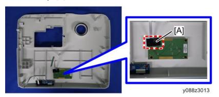
3. Remove the FFC cable [A]. (\*\*\*\*\*1)
