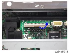
**10.** Insert the tab [A] of the bracket into the cutout, and attach the G3 interface unit [B].
