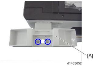
12. Make two loops with the telephone cord, and then attach the ferrite core [A] to the cable.
