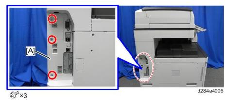
**2.** Remove the interface slot cover [A].
