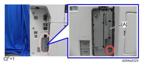
2. Insert the Fax Connection Unit SD card into SD card slot 1 [A: Upper Slot].
