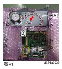
7. Attach the memory unit [B] to the FCU connector [A]
