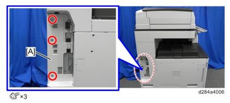
**2.** Remove the interface slot cover [A].
