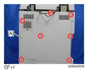
**3.** Remove the controller box cover [A].
