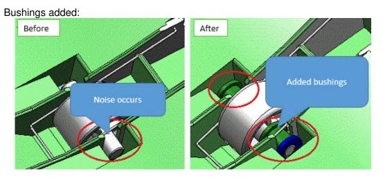
**IMPORTANT:** Due to the above changes, make sure to replace the cover, side guide plate, and roller shaft **together as a set.**
