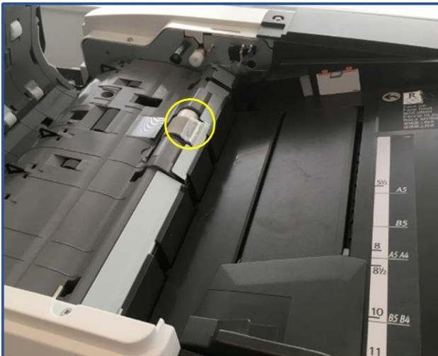
3. Remove the paper feed guide plate.
