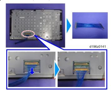
**<u>6.</u>** Remove the tapes for fixing the microphone harness (tape  $\times$ 3).
