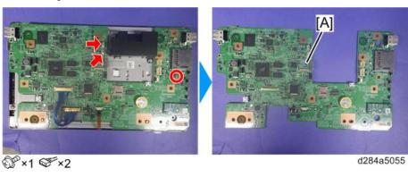
• By factory default, the following switches of the DIP switch [A] on the micro computer board are set to ON: No.1, No.3, No.6 and No.7. When installing the operation panel unit, make sure that the DIP switch
