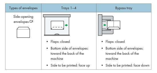
When loading envelopes, select "Envelope" as the paper types using both [Tray Paper Settings] and printer driver and specify the thickness of envelopes. For details, see "Printing on Envelopes", Print.
