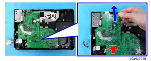
4. Remove the audio board [A] (@M3×10 Tapping screw×2, @\*×2).
