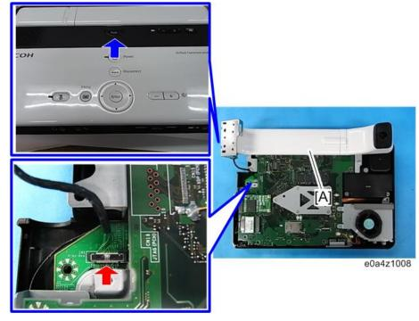
6. Push the "Push" button and remove the Camera unit [A] (😂 ×1).
