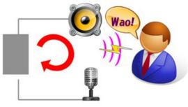
The common cause of acoustic feedback in a karaoke room or hall is illustrated below.
