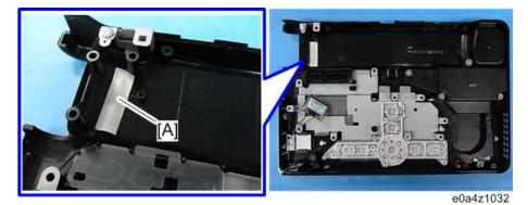
5. Remove the antenna modules [A].
