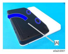
2. Remove the loss prevention strap [A] and remove the battery cover (  $\mathscr{F} \times 1$  )
