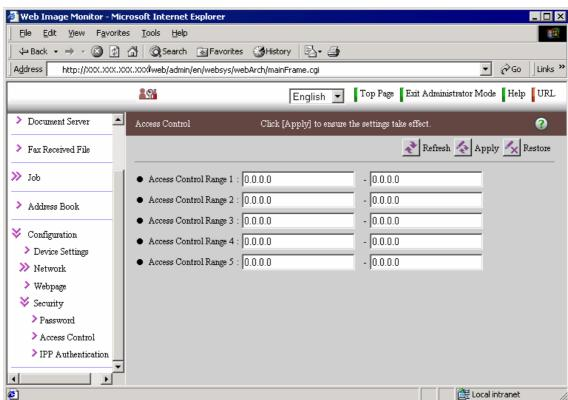
(4) To open the access control settings, click 'Configuration' -> 'Security' -> 'Access Control'.
