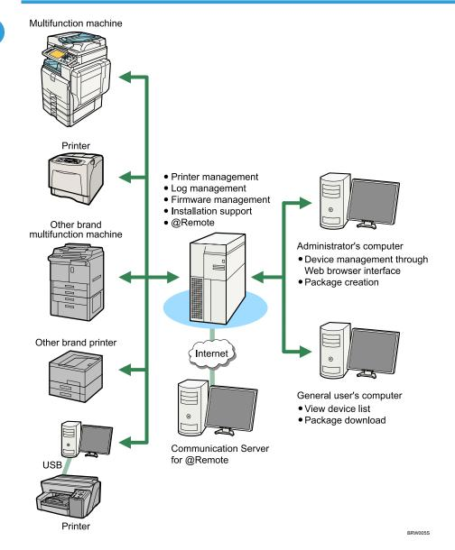
To use the @Remote service, Remote Communication Gate S Pro @Remote Connector is required. For details, contact your service representative.
