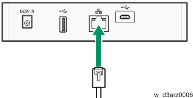
Connect this appliance to the network with the supplied network cable. You can use 10BASE-T, 100BASE-TX or 1000BASE-T network cable instead of the supplied cable. When connecting to the network via a 100BASE-TX or 1000BASE-T network cable, use a Category 5 or higher cable.
