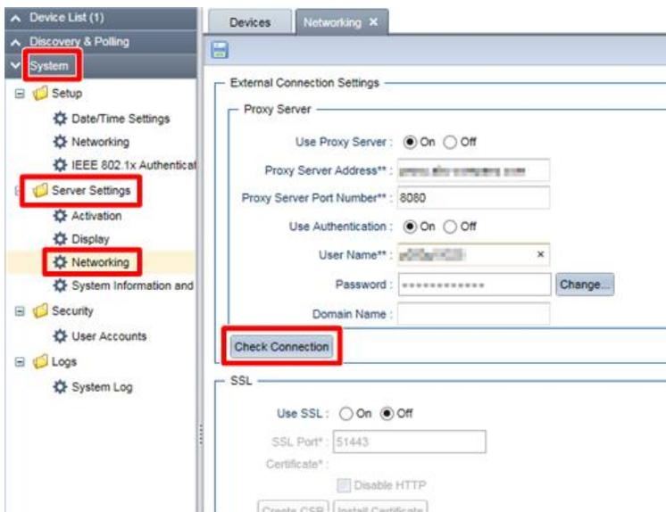
4. Check if the IP addresses of the proxy server and the DNS server are correct.
