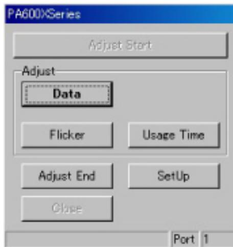
\* When Usage Time Data is written, it is necessary to turn the power supply ON (for one minute) after data writing. Turn the projector power supply ON.
