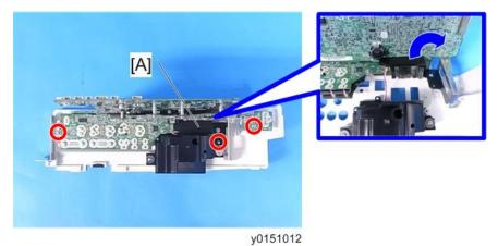
4. Remove the bracket [A] ( \*x3).
