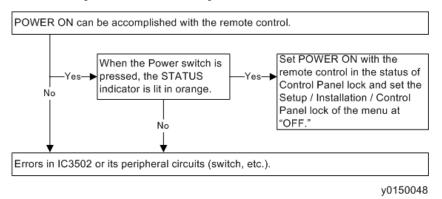
2. Normal video display is not presented with the COMPUTER1/COMPUTER2 (ANALOG) input (RGB/Component).
