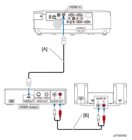
[A]: HDMI cable (not supplied) Use High Speed HDMI® Cable.
