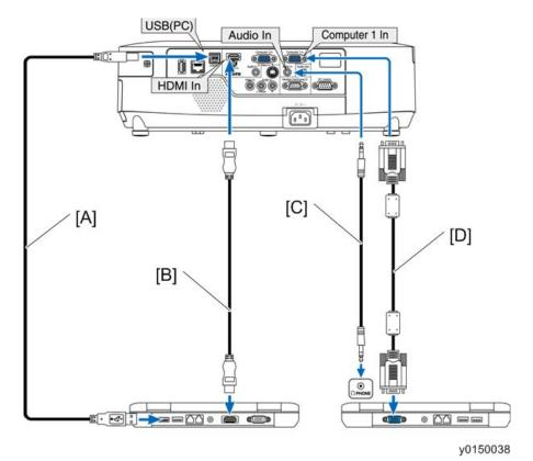
[A]: A commercially available USB cable (compatible with USB 2.0 specifications)
