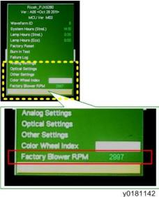
6. Check the value of "Factory Blower RPM". It should be from 2880 to 4320 rpm.
