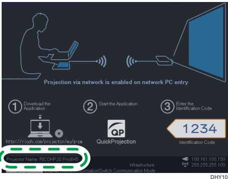
5. On the DLNA-compatible device, select the projector name checked in Step 3 as a destination device.
