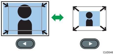
Press the [◀] button to reduce the size of the projected image. Press the [▶] button to enlarge the size of the projected image. The image is enlarged until it reaches the original size.
