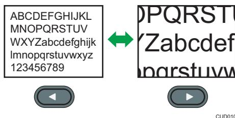
Press the [◀] button to decrease the magnification ratio. Press the [▶] button to increase the magnification ratio.
