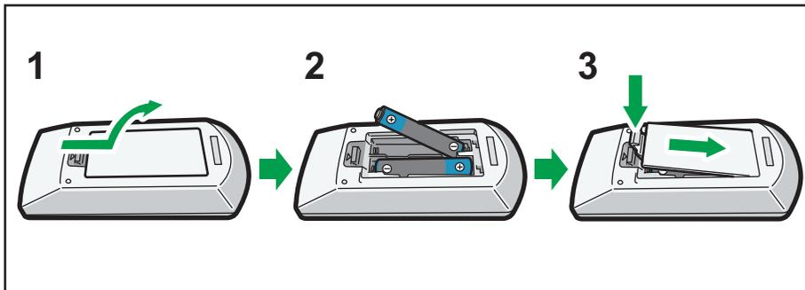
**1. Remove the battery cover from the remote control.**
