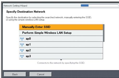
3. If you select **[Manually Enter SSID]** in Step 2, enter the SSID, and then press the **[Enter]** button.
