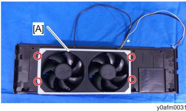
2. Remove the fan 2 and 3 from the fan bracket [A].
