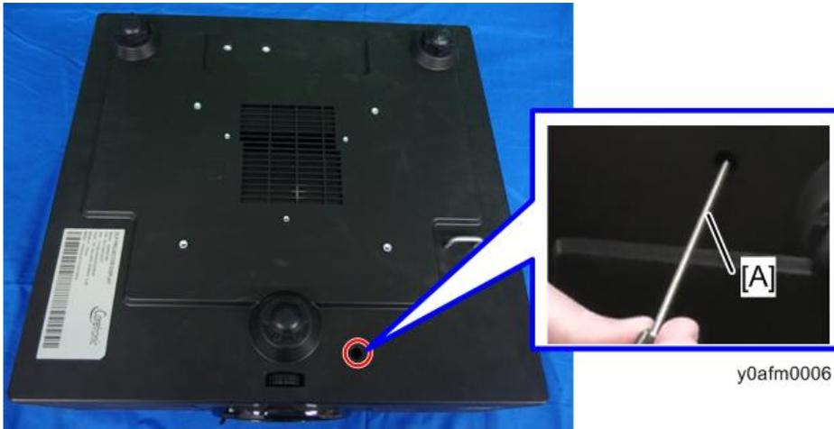
2. Remove 3 screws on the back cover (🔩 x3).
