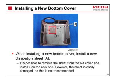
The spare part for the bottom cover does not have the dissipation sheet attached. So, if you need to install a new cover, you must order a new dissipation sheet also.
