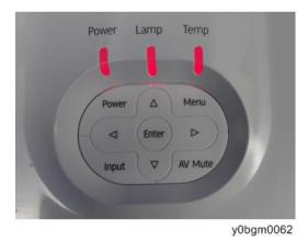
2. After all LEDs light red, as shown in the photo below, release the "Power" key.
