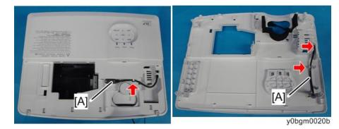
2. Pull out the mini HDMI Cable [A] from the top cover [B].
