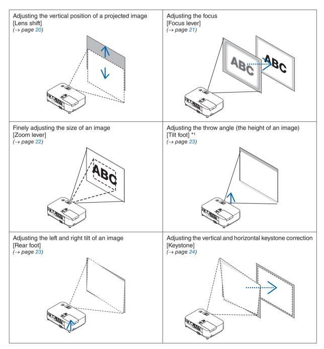
NOTE\*1: Adjust the throw angle (the height of an image) when the image position is higher than the lens shift adjustable range.
