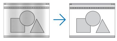
FREQUENCY ........ Use this item to fine tune the computer image or to remove any vertical banding that might appear. This function adjusts the clock frequencies that eliminate the horizontal banding in the image. This adjustment may be necessary when you connect your computer for the first time.
