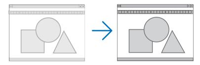
PHASE ...... Use this item to adjust the clock phase or to reduce video noise, dot interference or cross talk. (This is evident when part of your image appears to be shimmering.) Use [PHASE] only after the [FREQUENCY] is complete.
