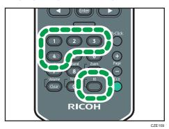
After the ID number of the remote control is switched, you can operate the projector with the remote control.
