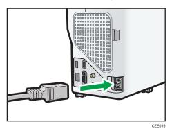
2. Insert the power plug into a power outlet.
