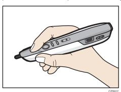
To align the point position of the electronic pen with the pen nib switch, and not the center of the pen, use the point adjustment button to move the point position up.
