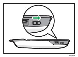
2. Push down A and slide the battery cover to remove it.
