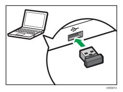
When the registered computer USB adapter is installed into the computer, the adapter flickers once every 0.5 seconds. Then, when the computer USB adapter is connected to the projector, the adapter flickers once every two seconds. If the adapter flickers twice every 0.5 seconds, you need to register it on the projector.
