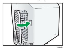
Insert the left side of the air filter in first, and then press the lever while pushing in the right side of the filter.
