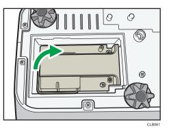
4. Hold the handle, and then pull the lamp unit out of the projector.
