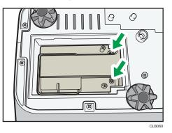
Make sure that the small projections inside the projector are inserted into the holes of the lamp unit properly.
