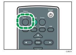
The input signal is detected automatically and the image is projected. The input signal changes each time the [Input] button is pressed.
