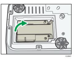
4. Hold the handle, and then pull the lamp unit out of the projector.
