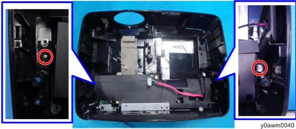
7. Turn over the tape [A] that fixes the bottom cover, and remove the PSU unit [B] with the bottom shield plate.
