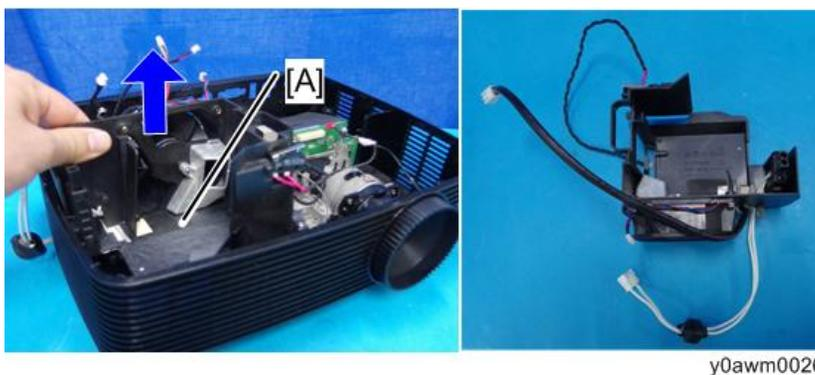
7. Release the connector for lamp module [A] from the lamp housing (M2.6 x7
