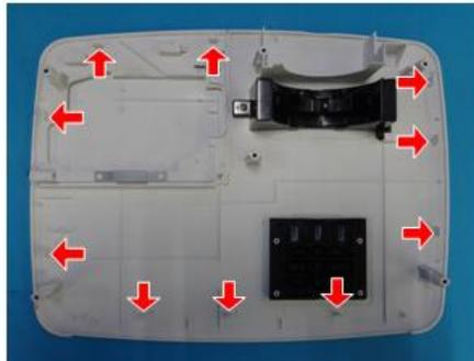
3. Place the top cover upside down, and remove the zoom lever [A] and keypad rubber [B] (M3 x6 ⚙️ x1).
