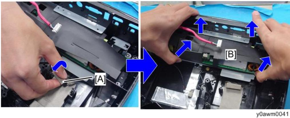
8. Open the insulating sheet of the PSU unit.
