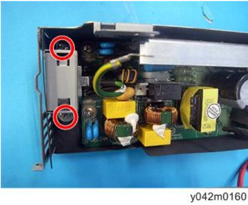
4. Remove the 5 screws and 2 connectors to separate the LVPS [A].
