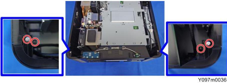
3. Remove 6 screws (red circles) and 8 hex screws (yellow circles) on the back side (🔩 x14).
