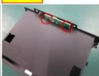
Fan 9 is at the left side of optical engine, and behind the CHIP PCB.
