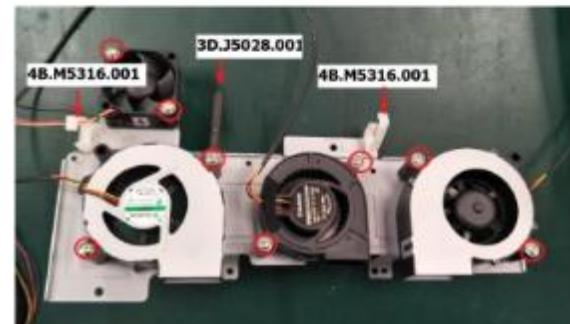
Fan 3,4: Open the back cover and take out the module. Fan detector PCB is on the module.
