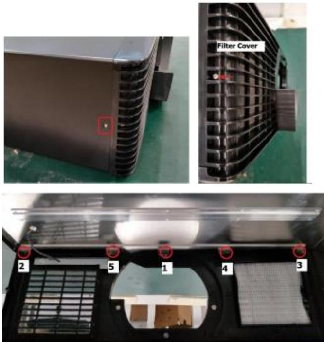
3. Remove the connector and all the screws and take out the front IR · LED PCB.
