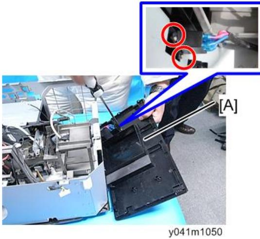
2. Remove the 2 screws to remove the lamp cover [A].
