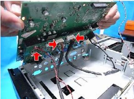
2. Remove the 3 screws to remove the GEO dummy board [A].
