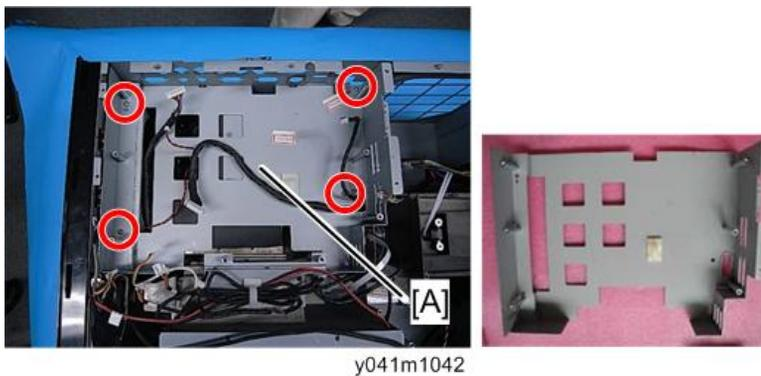
2. Remove the 2 screws to remove the front shielding [A].
