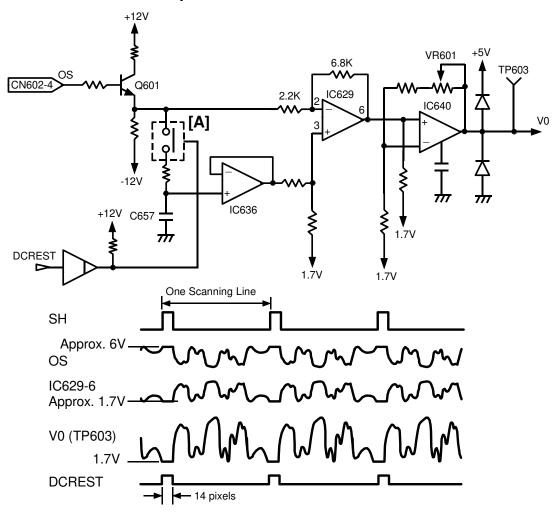
The analog signal (OS) from the CCD is output to the A/D conversion PCB. It is sent in the minus direction under the dc bias voltage (approximate 6 volts).
