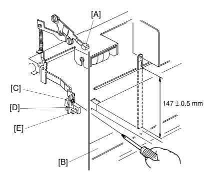
**Purpose:** To ensure smooth paper feed. **Adjustment Standard:** 147 ± 0.5 mm
