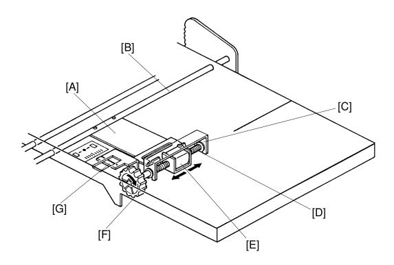
The shaft [D] of the fine adjusting dial [F] is threaded. The inside of the sleeve [E] is also threaded. The sleeve is fixed to the paper table stay [B] through a bracket [A].
