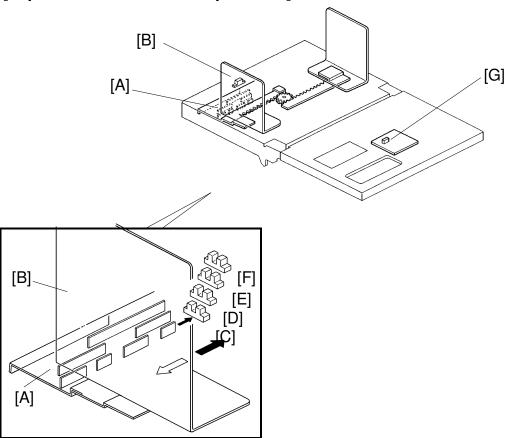
The paper width detection plate [A] installed behind the front paper side guide [B] has several interrupters.
