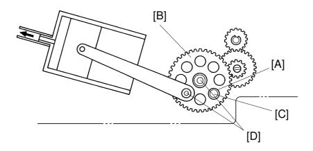
**Purpose:** To ensure that the paper exit pawl air pump produces a jet of air when the paper exit pawl is in the upper position (near the drum surface).
