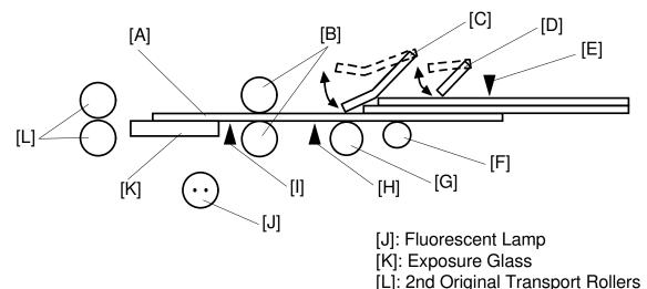
Two original feed modes can be selected by the ADF ON/OFF select switch.
