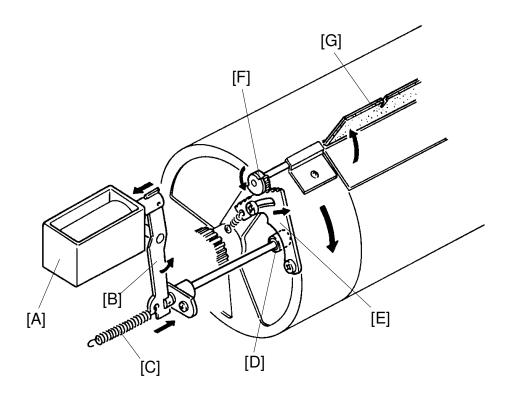
When the drum rotates 306 degrees (in reverse) past the home position, the master eject clamper solenoid [A] turns on and lever [B] rotates counterclockwise as shown. This moves the cam [D] inside the drum. Drum rotation brings the clamper sector gear [E] against the cam [D]. Gear [F] turns counterclockwise as it engages the clamper sector gear, thus opening the master clamper [G]. This releases the master from the drum.
