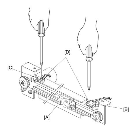
**Purpose:** To ensure that the cutter slider stops properly. **Adjustment Standard:** Confirm that the cutter holder activates the switches.
