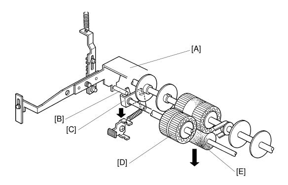
When printing is finished or a misfeed occurs, the paper table drive motor rotates for 500 milliseconds to lower the paper table. The paper on the paper table moves down from the paper feed roller [D] and the paper feed bracket [A] is pulled down by its own weight.
