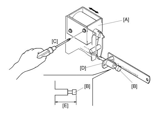
**Purpose:** To ensure that the master feed clamper is open during the master feed process and is closed during other processes.
