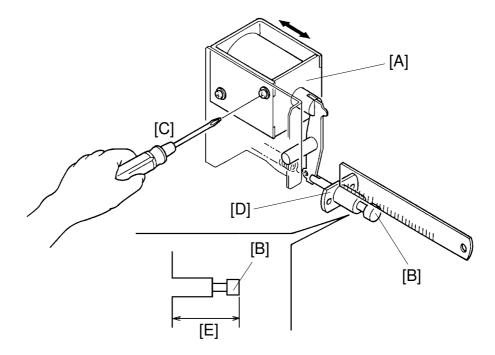
**Purpose:** To position the master eject clamper cam [B] so that the master clamper opens correctly during the master eject process and closes correctly for all other processes.
