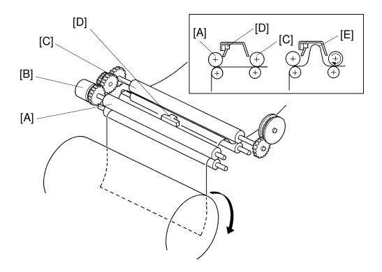
When the magnetic clutch [B] is turned off, the reverse roller [A] stops.
