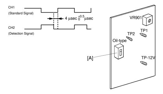
**Purpose:** To ensure that the ink detection PCB detects a no ink condition when the ink is running out.
