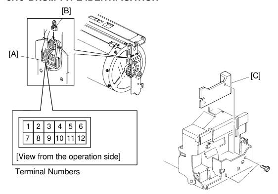
The machine identifies the drum type electrically. Depending on which terminal of the drum unit connector [A] is connected to, the corresponding indicator lights up on the operation panel as follows:
