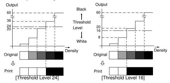
The binary processor converts 6-bit image data to single-bit white or black data to send it to the thermal head. This processor is used only for the line mode. (The binary processing for the photo mode is done by the half-tone processor.)
