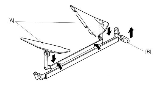
The wing guide[A] lifts up the sides of the paper as it exits the machine.
