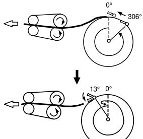
T4: When the drum rotates 13 degrees past the drum home position, the drum stops rotating.
