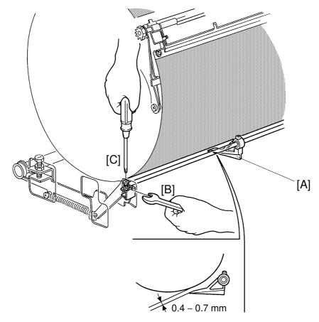
**Purpose:** To ensure that the printing paper is delivered without a paper wrap problem or damage to the screen.
