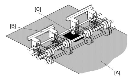
**Purpose:** To ensure that the sensor detects the ejected master. **Adjustment Standard:** 0.8 to 0.9 V when no master is detected.
