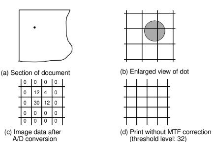
Consider a small black point on a original as shown in the illustration (a) and (b). The 6-bit image data (range 0 to 63) for this section of the original is shown in (c). If the threshold level is 32, all the pixels in this area will becomes single-bit white data and the image will not be reproduced (d).
