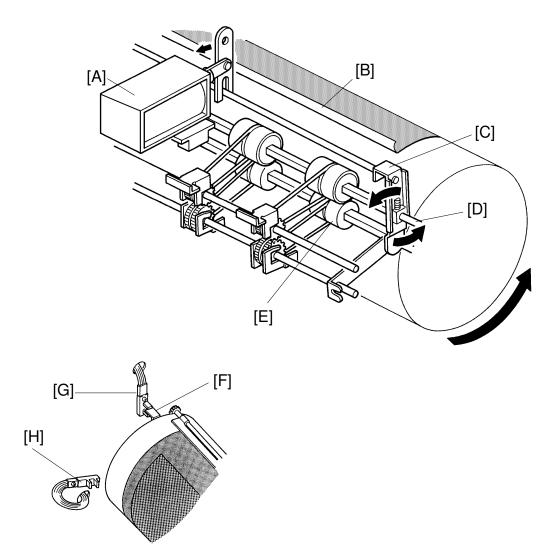
The drum position is detected by the first [G] and second [H] drum position sensors. When the drum reaches its home position, the first drum position sensor [G] is activated by the interrupter [F] at the rear side of the drum.
