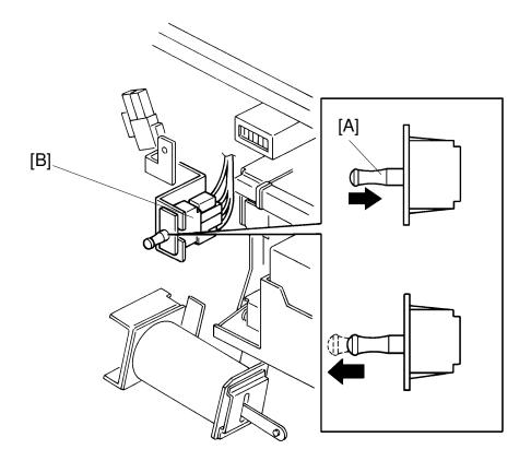
Pull out the actuator [A] of the interlock switch [B] located inside of the inner cover to disable the front door, paper table, master eject unit, and scanner unit safety switches. The interlock switch remains activated as long as the actuator is pulled out.
