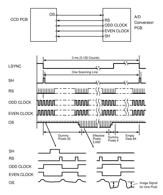
The light reflected from the original exposes the CCD (Charge Coupled Device). The CCD is a solid-state device similar to a photodiode array, but unlike a photodiode array, a CCD can read one complete scanning line at a time.
