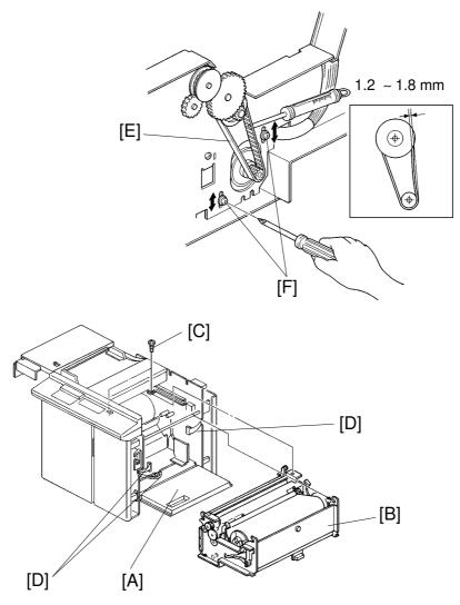
**Purpose:** To ensure that proper rotation for the master feed is transmitted to each roller.
