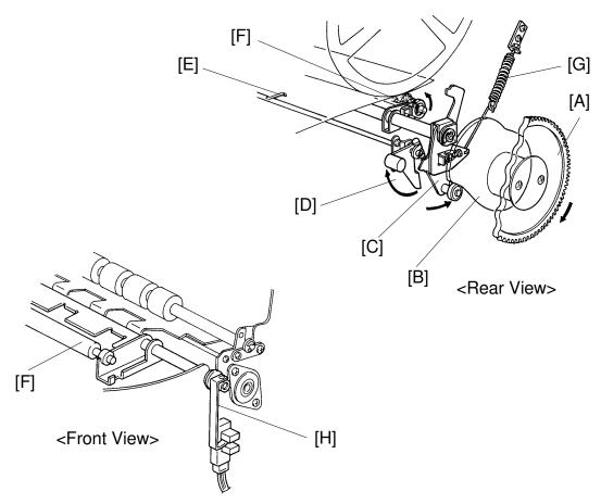
During the printing process, the main motor turns the gear [A] and pressure cam [B] clockwise.
