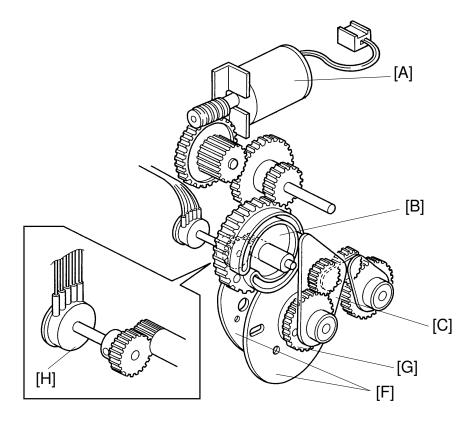
In image positioning mode, the image can be shifted 20 mm (5 mm steps) up or down on the page by pressing the forward or backward Image Position key on the operation panel. This rotates the first and second paper feed roller cam to change the paper feed timing in relation to the drum rotation timing.
