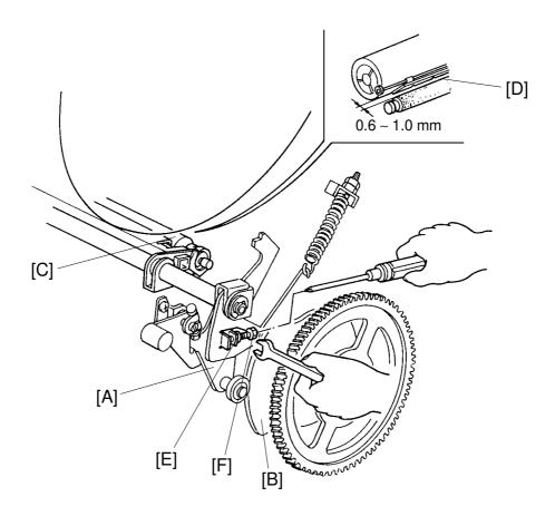
**Purpose:** To ensure that the press roller does not touch the clamper section of the drum.
