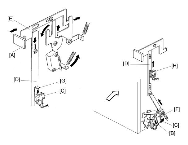
The master eject open button [A] locks when the paper delivery table is closed. This lock mechanism functions as follows:
