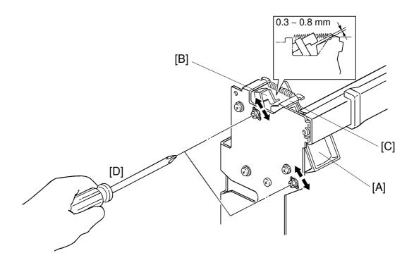
**Purpose:** To ensure that the drum can be removed only when it is in the home position.
