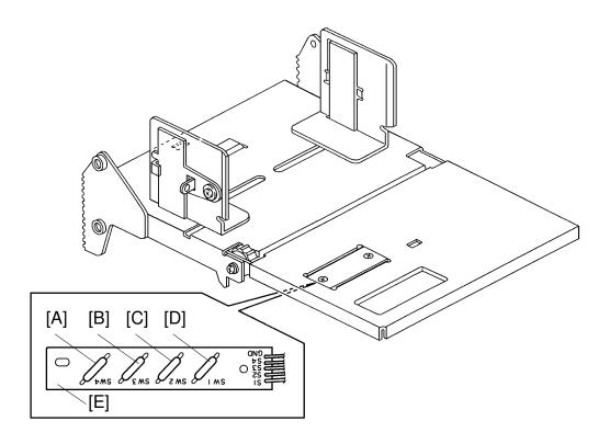
The machine determines the cassette size through the cassette size detection PCB [E]. The reed switches on this PCB are activated by magnets positioned on the back of the cassette. The magnets are positioned according to the paper size (the magnet position for each of size paper is described on the back of the cassette). Depending on which reed switches [A] [B] [C] [D] are activated, the machine determines the cassette size as shown in the table below:
