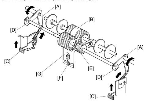
Spring tension [F] holds the separation plate [G] against the upper separation roller. A rubber pad is on top of the separation plate to separate a few sheets of paper before they reach the lower separation roller. If too many sheets of paper are fed to the lower separation roller at the same time, the lower separation roller will maybe not separate the sheets, it can separate only two or three sheets of paper.
