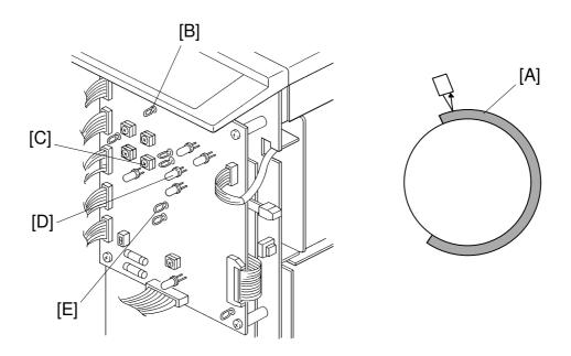
**Purpose:** To ensure that the drum master detection sensor correctly detects the master on the drum.
