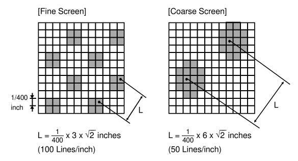
In this model a  $12 \times 12$  dither matrix is used to convert 8-bit image data into single-bit data. There are two kinds of dither matrices to allow for the fine and coarse screen modes.
