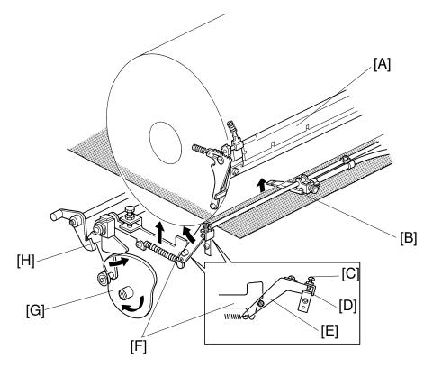
The exit pawl [B] located in the center of the drum, guides the center of the printing paper. As the master clamper [A] approaches the exit pawl, the exit pawl moves away from the drum.
