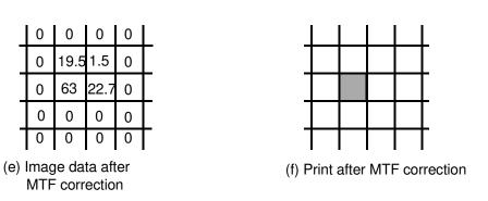
After the MTF correction is applied, the image data of the example is as shown in (e) and (f) above. The small black point is reproduced on the print.
