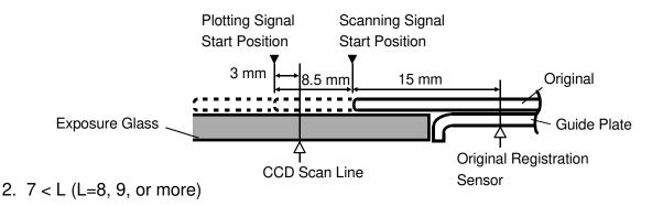
When the shifting length L is longer than 7 millimeters, the image of the original is moved backwards by advancing the master feed timing in the master making process.
