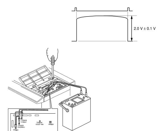
**Purpose:** To set the white level so that the background of the test chart is not copied.
