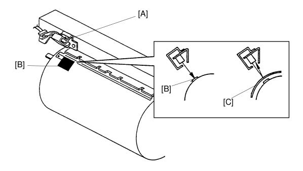
The drum master detection sensor [A] is mounted on the drum rail and it detects whether a master is on the drum.
