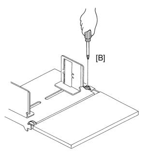
**Purpose:** To ensure that the paper table open switch turns on to prevent the paper table from going up when the paper table is closed.
