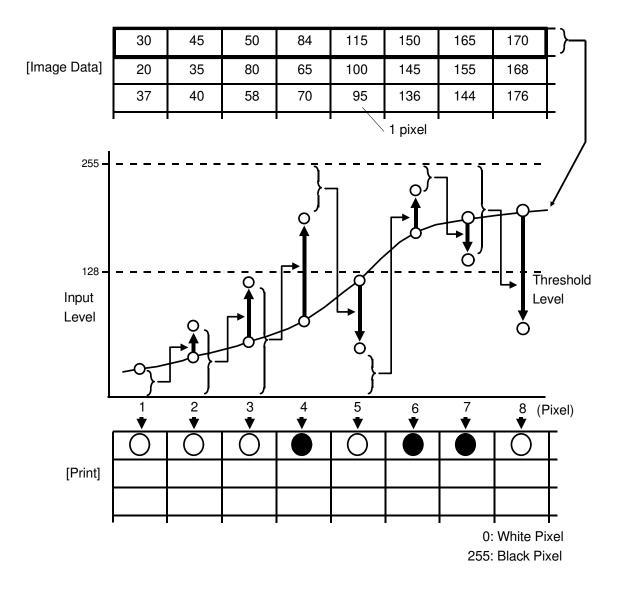
In this model, the errors are distributed in three dimensions. The error is preferentially distributed to darker pixels in higher ratio and to lighter pixels in lower ratio. CAPIX has the following advantages:
