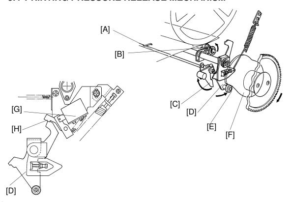
The pressure release solenoid [G] energizes to release the pressure ON/OFF lever [D] when the paper feed solenoid energizes during normal operation.
