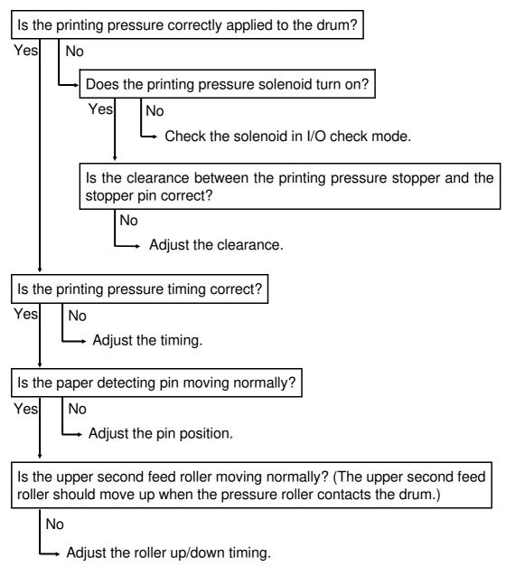
4. Paper frequently jams or is not fed during high speed printing. (Does not occur at low printing speeds.).
