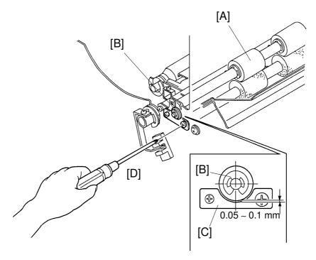
**Purpose:** To ensure that paper is fed straight between the drum and the press roller.
