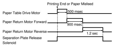
When the paper feed stops, there may still be some paper between the upper and lower separation rollers. This mechanism returns any paper between the rollers back to the paper stack on the paper table.
