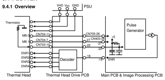
A thin-film type thermal heating element is used by the thermal head. The thermal heating elements melt the over-coating and polyester film layers of the master according to the image signals for each pixel. The specifications are as follows:
