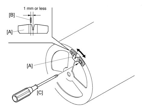
**Purpose:** To ensure that the drum is securely locked when the drum unit is pulled out.
