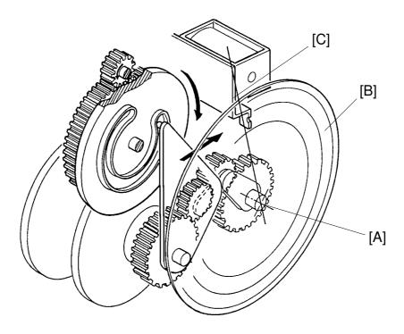
**Purpose:** To ensure paper feed by regulating the timing to start the second feed roller.
