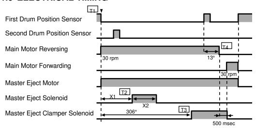
T1: When the Master Making key is pressed, the main motor and master eject motor start turning. At the same time, the paper table drive motor starts turning to lift the paper table to the paper feed position.
