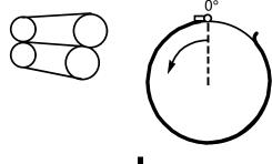
T2: When the drum rotates X1 degrees past the first drum position sensor actuation position (drum home position), the master eject solenoid is energized. This presses the lower eject rollers against the drum surface. The master eject solenoid is de-energized when the drum rotates X2 degrees more.
