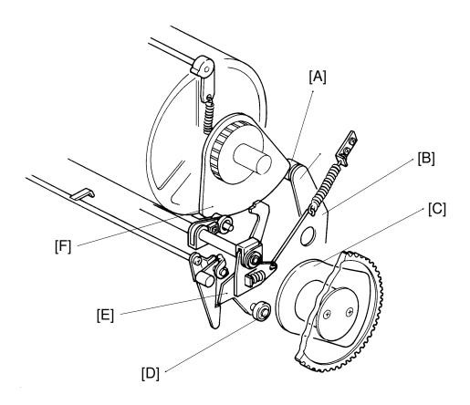
When the A3/DLT drum is used, printing pressure is applied while the bearing [D] of the pressure ON/OFF lever [E] is on the bottom of the pressure cam [C]. Pressure is released while the bearing is on top of the cam.
