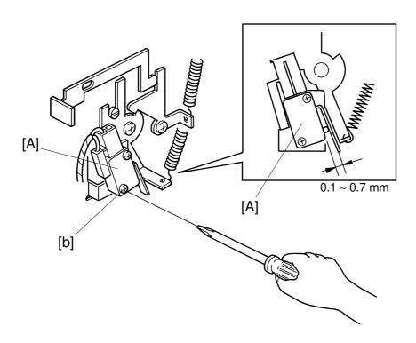
**Parpose:** To ensure that the safety switch turns on and stops the air knife motor when the master eject unit is opened.
