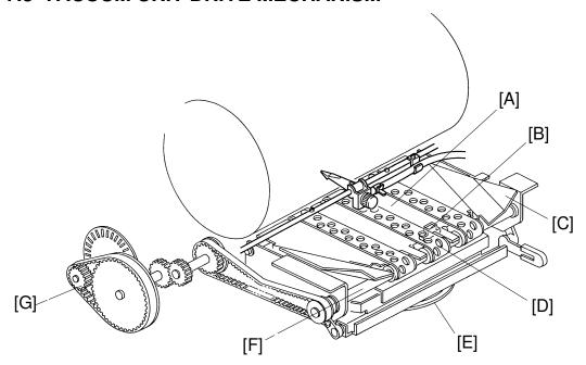
The vacuum fan [E] holds the paper against the transport belts [D]. The transport belts move the paper to the delivery table.
