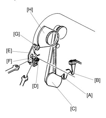
**Purpose:** To keep the distance between the press roller and the drum constant while the printing pressure is released.
