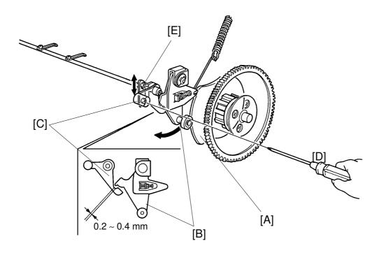
**Purpose:** To ensure that printing pressure is applied during paper feed, and is released correctly afterwards.
