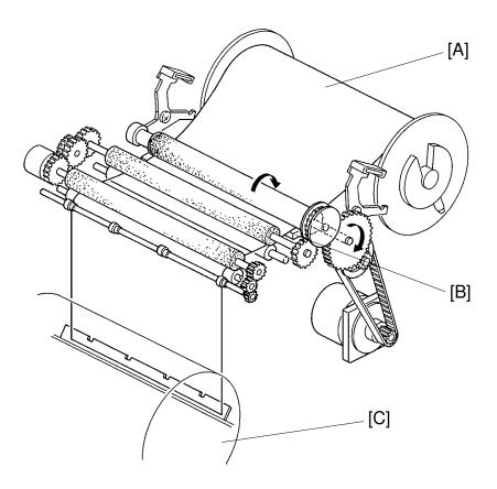
The thermal head [B] burns the image (scanned by the CCD) on the master [A] as it is being fed to the drum [C]. The master is then clamped to and wrapped around the drum.
