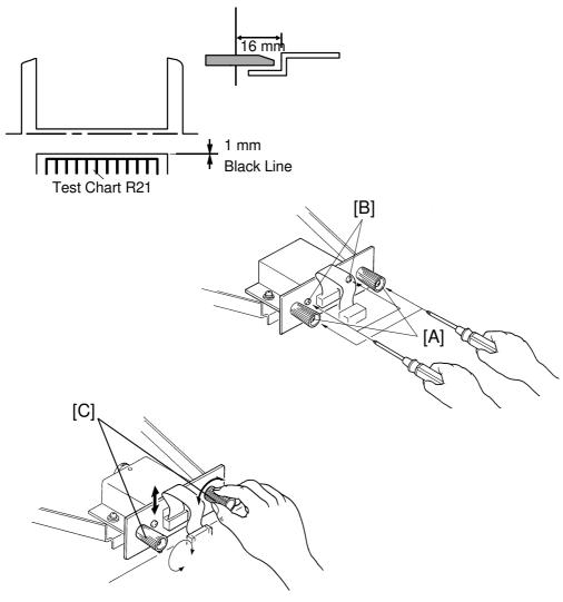
**Purpose:** To ensure that the CCD alignment is perpendicular to the original feed direction.
