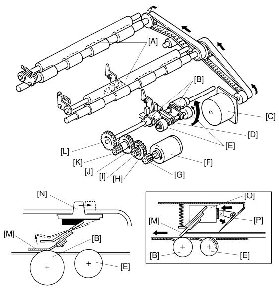
The original transport rollers [A] are driven by the original transport motor [C], which is a stepper motor. The original feed rollers [B] are driven by the ADF drive motor [F] (dc motor) through a series of gears [G] to [L]. The pull-out rollers [E] are driven by the ADF motor through a drive belt [D].
