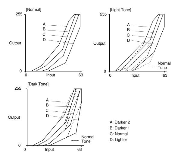
The compensation ratio varies according to which image density and contrast are selected. For example when Darker 1 key is selected the output value of the image data is increased slightly (i.e. it is slightly higher than the output obtained when Normal density is selected).
