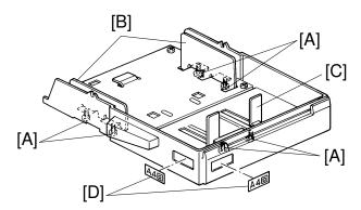
2. Move the 3 fences to the desired paper size position and tighten the 6 screws.
