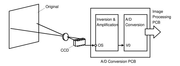
This system converts analog image data into digital form. It then alters the data to correct for image intensity distortions caused by uneven light intensity.
