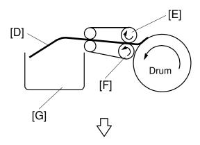
The trailing edge of the master curls off the drum and passes between the upper [E] and lower [F] eject rollers, and the master [D] is dumped into the master eject box [G].
