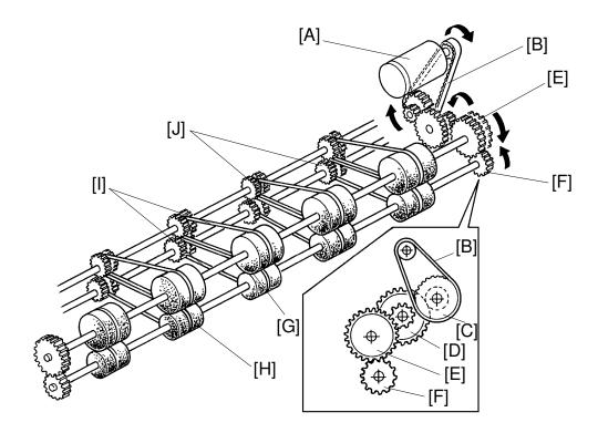
When the original is set and the Master Making key is pressed, the main motor starts turning at 30 rpm in reverse. So now the drum also turns in reverse (compared with the printing rotations).
