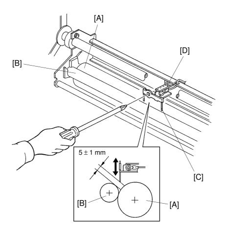
**Purpose:** To ensure detection of ink built-up between the ink roller and the doctor roller.
