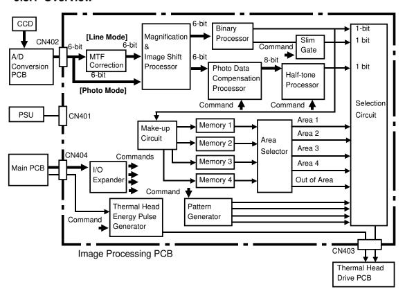
The upper 6 bits of the 8 bits from the A/D conversion PCB are used by this board. (The other 2 bits are not needed and are discarded.) The digital data are inverted to match with the circuit of the image processing PCB. Therefore, the white peak level becomes 0, and the black peak level becomes 63.
