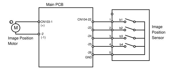
When the forward Image Position key is pressed, CN103-2 goes to 22 V and CN103-1 goes to 0 V, and the image positioning motor turns to advance the paper feed timing.
