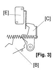
When the drum unit is set in the machine, the arm [B] is pushed by the lock pin [D] until the top of the arm [B] is locked by the stopper [C]. The lock pin [D] is mounted on the front side plate of the main body. This completely locks the drum unit in the machine (Fig. 1). At the same time, the top of the right stopper [C] turns on the drum detection switch [E]. The switch [E] tells the machine that the drum unit is set (Fig. 3).
