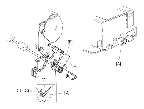
**Purpose:** To ensure that the second feed roller starts rotating when the paper feed solenoid turns on and stops rotating when the paper feed solenoid turns off.
