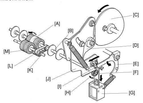
The sector gear [J], located on the non-operation side, rotates the paper feed roller [M] and the upper separation roller [A]. When the paper feed solenoid [G] turns on, the link [F] is pulled. When the cam roller [D] is positioned on top of the paper feed roller cam [C], the sector stopper [E] turns counterclockwise as a clearance is formed between the pin [I] and the stopper [E]. Then, the cam roller [D] of the sector gear moves along the cam face of the paper feed roller cam [C].
