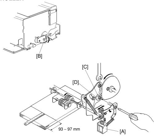
**Purpose:** To ensure paper feed to the second paper feed roller. **Adjustment Standard:** 93 to 97 mm
