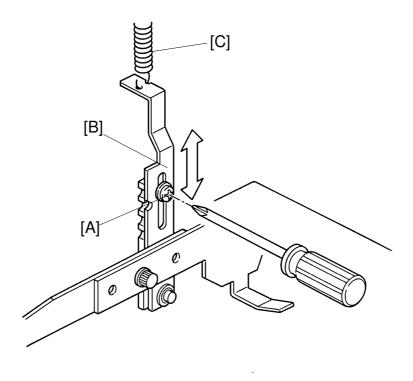
**Purpose:** To ensure that the paper feed roller exerts sufficient pressure for a smooth paper feed (printing paper weight range of 50 g/m<sup>2</sup> to 215 g/m<sup>2</sup>).
