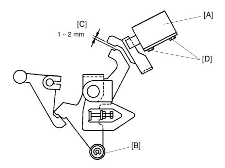
**Purpose:** To ensure that the printing pressure stopper is released when the paper feed starts, and that the stopper is locked within one drum rotation when a paper jam occurs.
