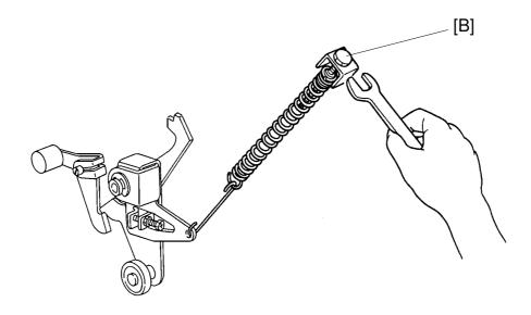
**Purpose:** To apply the proper printing pressure to the press roller. **Adjustment Standard:** 4 mm
