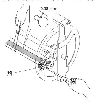
**Purpose:** To equalize the ink thickness around the ink roller and prevent an uneven image.
