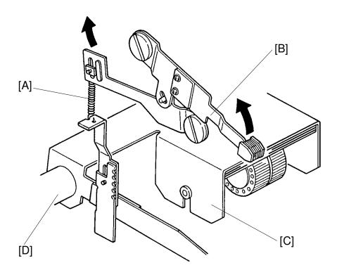
Due to the weight of the feed roller assembly [C] the paper feed roller presses the paper stacked on the paper table. This is because the feed roller assembly rotates freely around its shaft [D].
