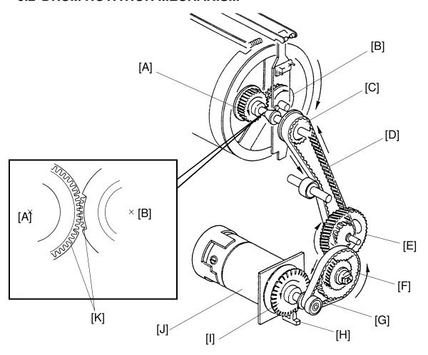
The main motor (DC motor) [J], located under the rear side plate, turns the drum either clockwise or counterclockwise through belt [G], then through gears [F] and [E], then belt [D], and pulley [C]. The drive mechanism uses helical gears because they turn more quietly.
