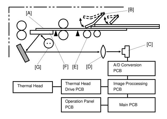
The first original [A] at the bottom of the stack on the original table is separated from the other originals by the original feed rollers [E] and the separation blade [B], and is fed onto the exposure glass [F].
