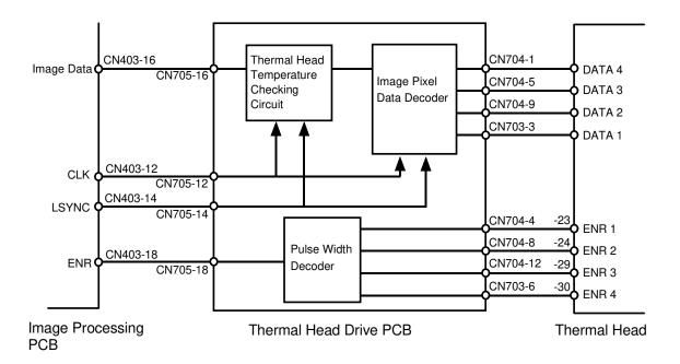
A thermal heating element may get too hot when there are consecutive black pixel data in the sub-scanning direction. Conversely, a thermal heating element may not get hot enough to plot on a master when there are consecutive white pixel data in the sub- scanning direction.
