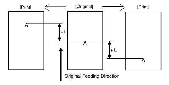
The image is shifted in the sub-scanning direction by changing the start timing for the original feed or master feed. (In the main scanning direction, the image is shifted by changing the output timing of the image data in the image processing PCB. See "9.3 IMAGE PROCESSING PCB".)
