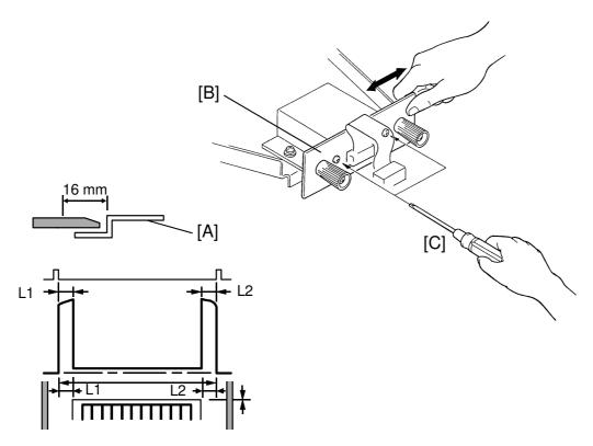
**Purpose:** To align the center of the original with the center of the CCD.
