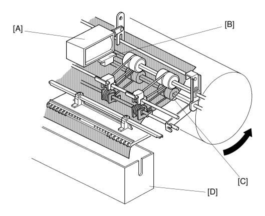
When the A3/DLT drum is 109 degrees from the home position, the master eject solenoid [A] turns off, separating the lower first eject rollers [C] from the drum.
