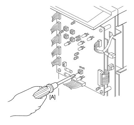
**Purpose:** To ensure the correct main motor speed.
