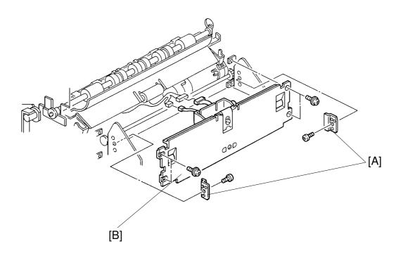
**Purpose:** To ensure that the separation plate is released from the upper separation roller when the paper table lowers.
