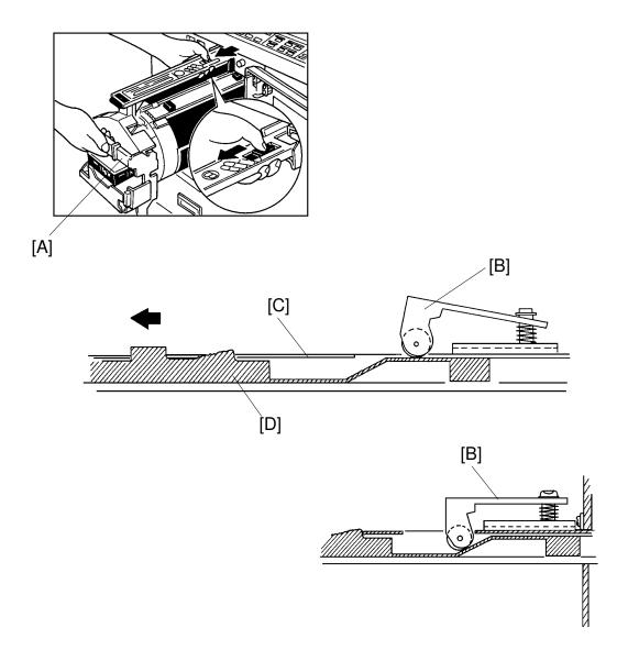
When the drum is pulled out, the drum stopper [B] drops in the hole (see above figure). This stops the drum unit from being pulled out any further. Now, if the operator pulls handle [A], the drum unit won't fall out.
