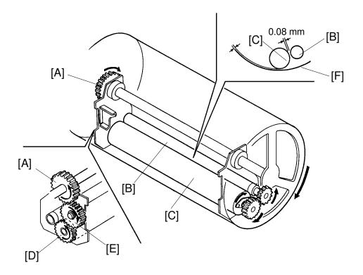
The ink kneading mechanism consists of the ink roller [C] and the doctor roller [B]. The ink roller [C] rotates with the drum and the doctor roller [B] insures that the ink goes evenly to the ink roller.
