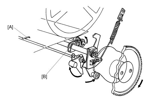
In this section, the paper detecting feeler [A] detects whether paper is fed correctly to the second paper feed roller section or not.
