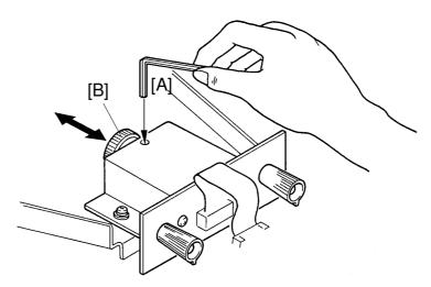
**Purpose:** To adjust the focus distance between the CCD and the lens.
