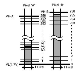
4. The digitized pixel data are sent serially to the image processing PCB. For example, data "A" (70) and "B" (255) are expressed in 8-bit form and sent through the eight terminals (BAD 0 to BAD 7) shown in the table on the right.
