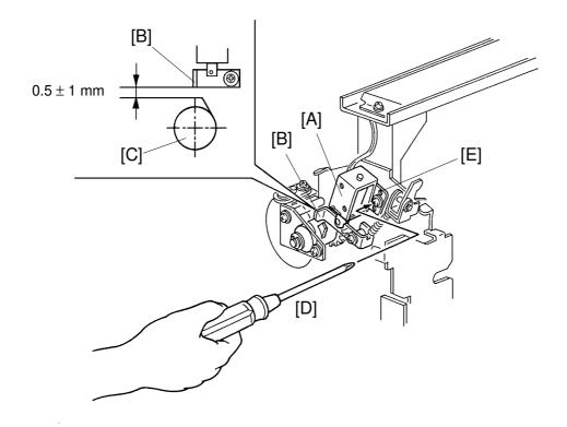
**Purpose:** To ensure total clutch-sleeve release by the stopper when the ink supply solenoid [A] turns on and complete clutch-sleeve locking by the stopper when the ink supply solenoid turns off.
