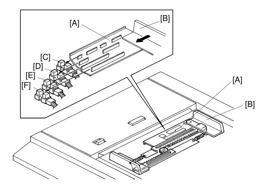
The original width detection plate [A] installed behind the rear original guide [B] has 4 photointerrupters.
