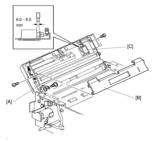
**Purpose:** To ensure that the originals are separated properly. **Adjustment Standard:** 6.0 to 6.5 mm
