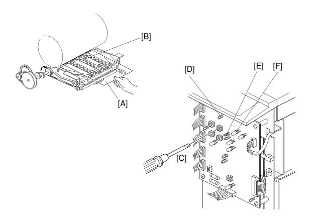
**Purpose:** To ensure that the sensor detects correct paper delivery, and to ensure that the jam indicator blinks properly after an exit misfeed or a paper wrap occurs.
