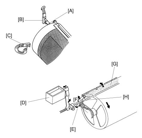
After the master eject process is finished and the interrupter [A] is positioned in the first drum position sensor [B], the main motor turns on and the drum starts rotating (30 rpm) in reverse (opposite to the printing direction).
