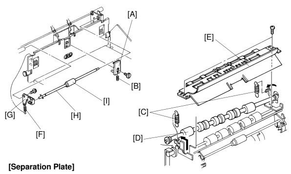
1. Remove the separation plate [A] with the spring [B] (1 screw).
