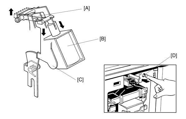
The drum lock solenoid [B] activates when the drum is turning. If someone interrupts the printing cycle by opening a cover, then the drum will stop. If the drum does not stop in the home position, then the drum lock will stay on. The stopper lock arm [A] then locks the left stopper [C] in place. This prevents the drum unit from being removed when it isn't in the home position.
