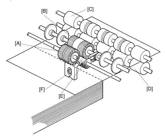
This mechanism uses a center separation system, which consists of the separation plate [F], upper separation roller [B], and lower separation roller [E]. Because of the separation system, if a few sheets of paper are picked up from the paper stack (paper table) by the paper feed roller [A], only one sheet of paper is transported to the second upper feed roller [C] and second lower feed roller [D].
