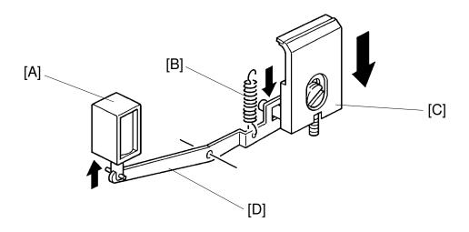
When the paper table starts going down, the separation plate release solenoid [A] is energized. The pressure release arm [D] turns clockwise, and the separation plate [C] moves down from the upper separation roller. This mechanism allows for easy removal of any paper caught between the upper separation roller and the separation plate.
