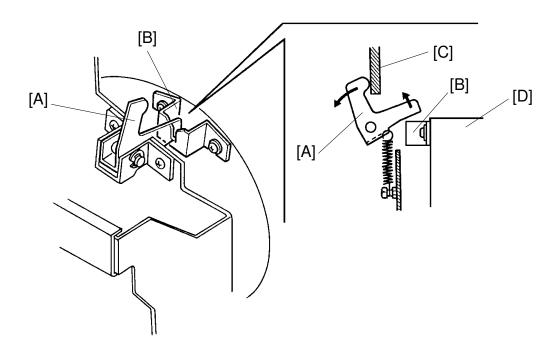
To prevent the drum from rotating when the drum unit is slid out, the drum stopper [A] drops into the drum lock [B]. This secures the drum [D].
