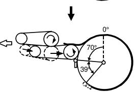
The drum rotation angles X1 and X2 depend on the drum type. This machine has two types of drums: one is the A3/DLT drum (standard), and the other is the A4/LT drum (optional). X1 and X2 for each drum are as follows:
