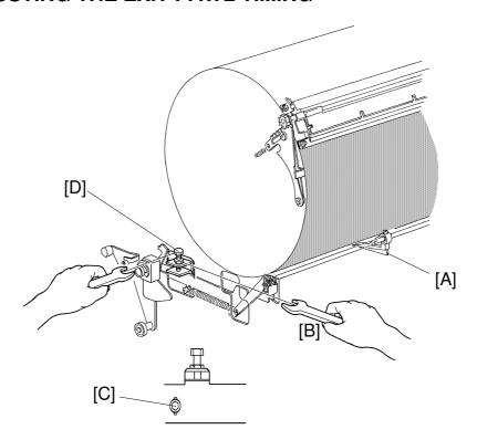
**Purpose:** To ensure that the exit pawl does not touch the master clamper. **Adjustment Standard:**  $232 \pm 3^{\circ}$
