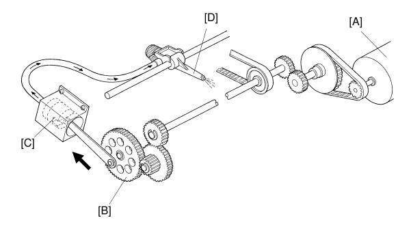
The main motor [A] turns a gear [B] through idle gears, a belt and a shaft. The gear [B] rotates and drives the piston [C] back and forth.
