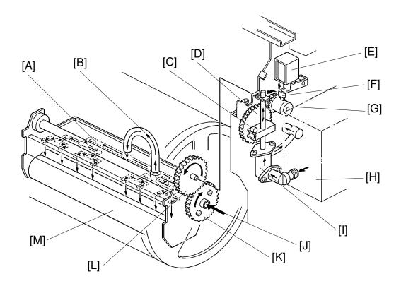
Ink is supplied from the ink cartridge [H] to the ink roller [M] by the ink pump [I] and then through 8 holes in the ink distributor [A].
