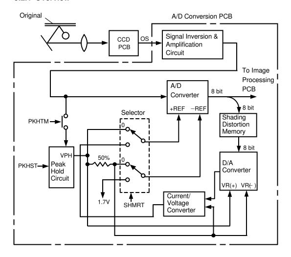
The analog signal generated from the CCD is inverted and amplified in the A/D conversion PCB. Then, the analog signal is converted into an 8-bit digital signal and is sent to the image processing PCB. The original background and the distortion of the light path are monitored to obtain the exact image data.
