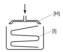
The pressure plate [H] compacts the ejected master [I].
