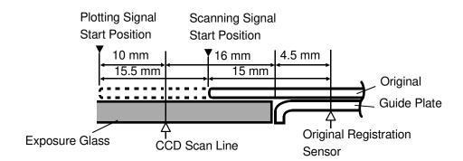
T1: When originals are inserted in the ADF unit, the first original sensor is activated.
