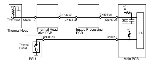
A thermistor on the thermal head and a thermal guard (a thermostat) on the power supply unit are used for thermal head protection. This prevents the thermal head and power supply unit from overheating when continuously processing a solid image. The CPU detects the abnormal condition and lights the SC code on the operation panel as follows:
