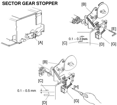
**Purpose:** To ensure that the paper feed roller starts rotating when the paper feed solenoid turns on and stops rotating when the paper feed solenoid turns off.
