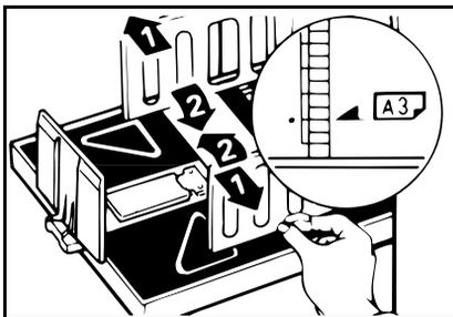
**6** Move the end plate until the plate handle is flush with the end of the table.
