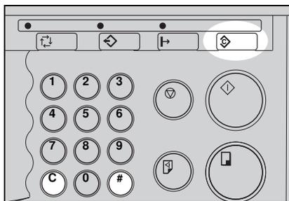
**2** "01" will blink on the Memory/Class indicators. Set the required service program number (SP No.) using the **Up** or **Down** key.
