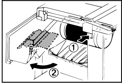
*When a master misfeed occurs in the master eject section*
