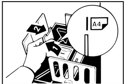
**9** If necessary, lift the left and right guides.
