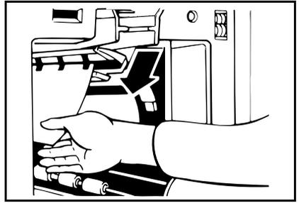
**5** If the original misfeeds in the optional document feeder, press the ADF open lever and open the ADF unit to remove the misfed sheet.
