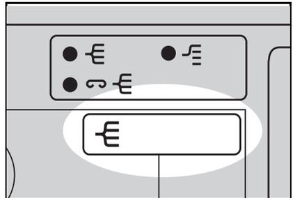
**2** If the Speed function Setting 1 indicator and the Special Feature indicator blink, set the speed to Setting 1.
