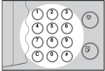
**4** Press the **Master Making** key. Check the image position of the trial or proof print.
