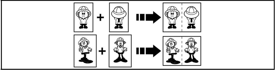
You can print 2 separate originals on a single sheet of paper. The following tables list the combinations that can be used when combining two originals.
