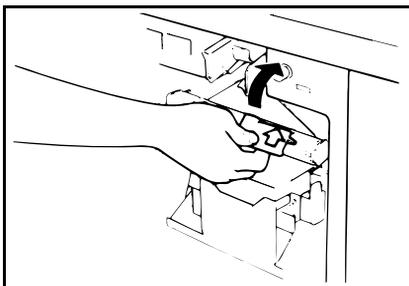
**4** Pull out the drum unit handle while pressing the release bar inside the green handle.
