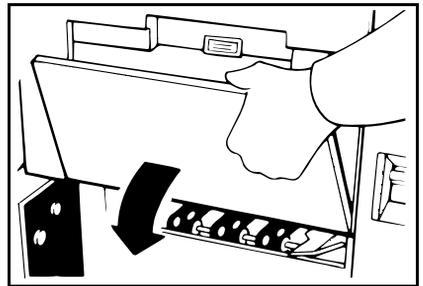
**2** Take out the master eject box and remove the used masters.
