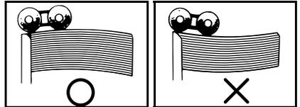
When the leading edge margin of the original is less than 5 mm, 0.2" or there is a solid image on the leading edge, insert the original with the widest margin first or make a leading edge margin by making a copy.
