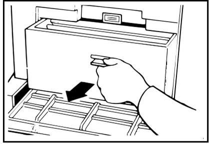
**3** Reinstall the master eject box. Push in the box until it touches the inside bracket.
