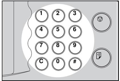
**5** Press the **Master Making** key. Check the image position of the trial or proof print.
