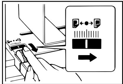
**2** Adjust the paper delivery side plates to the print paper position.
