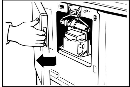
**2** Lower the ink holder and remove the used ink cartridge.
