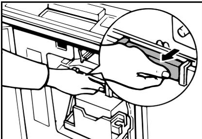
**5** Hold the rail on the drum and slide out the drum while pulling the release towards you.
