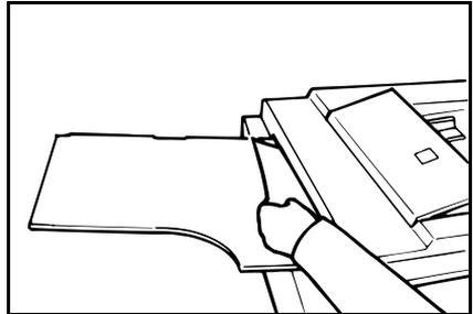
**4** If you still cannot remove the misfed paper, open the document feeder and remove the original.
