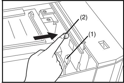
**8** Press the master cut button (2) to cut the leading edge of the master roll.
