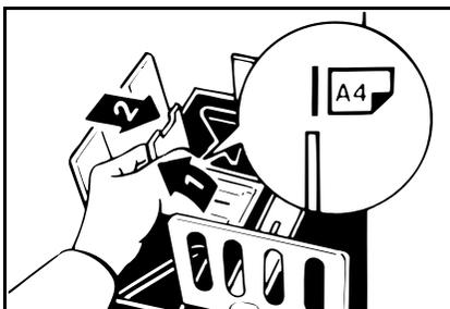
**10** If necessary, lift the left and right guides.
