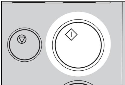
**6** Press the **Proof** key and check the image density and the image position of the proof print.
