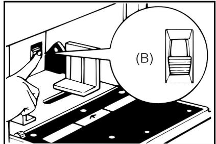
**3** Make sure that the wing guide release lever is upper position.
