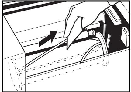
**6** Insert the paper edge of the master roll under the arrow mark (1) until you can see the leading edge under the transparent cover.
