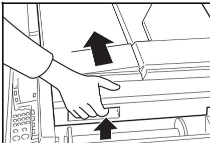
**2** Lift the pressure release lever in the direction of the arrow to release the feed roller pressure.
