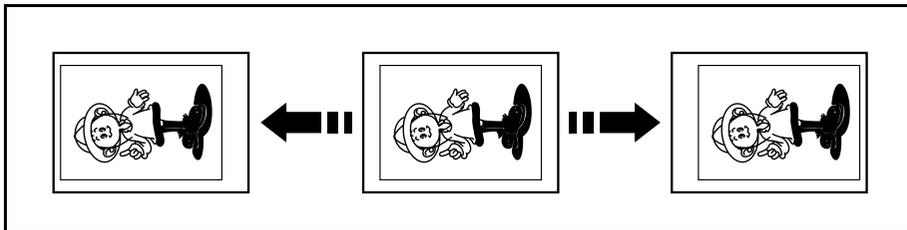
**1** Press the right **Image Position** key to move the image forwards, the left key to move it backwards.
