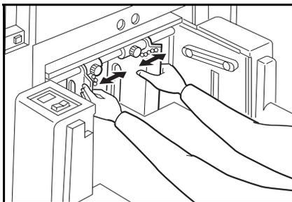
**7** Secure the side plates with the screws.
