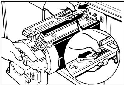
**6** Remove the drum unit from the machine while holding the upper drum stay.
