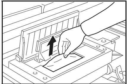
**4** If you could not remove the misfed master in steps **2** and **3**, take out the drum and remove the misfed master from the inside.
