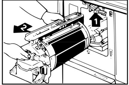
**2** Grasp the drum unit handle and remove the master from the drum.
