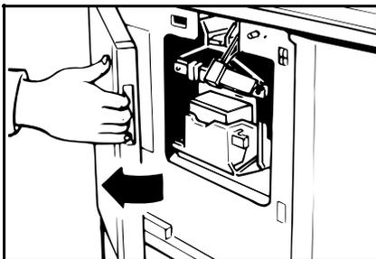
**2** Make sure that the lamp of the drum rotation button is green. If this lamp is red, press the drum rotation button until the beeper sounds and the lamp turns green.
