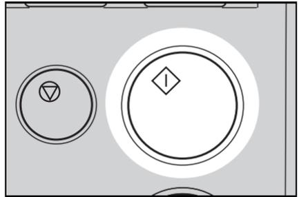
**10** The beeper sounds after the command sheet is scanned. Set the original face down on the exposure glass and press the **Master Making** key.
