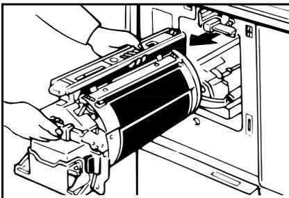
**7** Insert the color drum unit along the guide rail.
