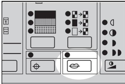
**2** Using the **Number** keys, select the Image Make-up mode for the first command sheet. (See page 4.)
