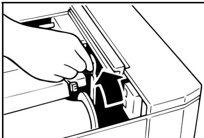
**3** Remove the used master roll and pull out both spools. Then, insert both spools into a new master roll.
