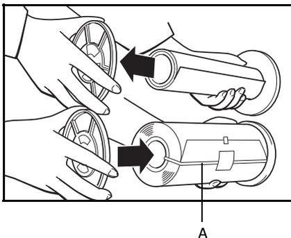
**4** The new master roll must be positioned as shown in the illustration.
