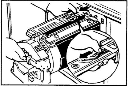
**6** Remove the drum unit from the machine while holding the upper drum stay.
