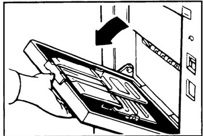
**7** Lift the paper delivery end plate and move it to match the print paper size.
