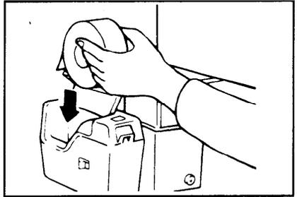
**3** Feed the leading edge of the roll in the dispensing slot until it stops.
