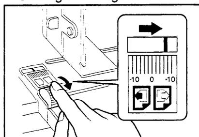
**2** Adjust the paper delivery side plates to the print paper position.
