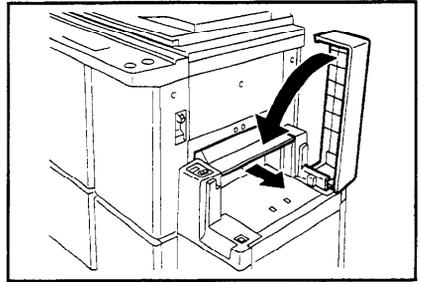
Make sure that the drum is completely set in position.
