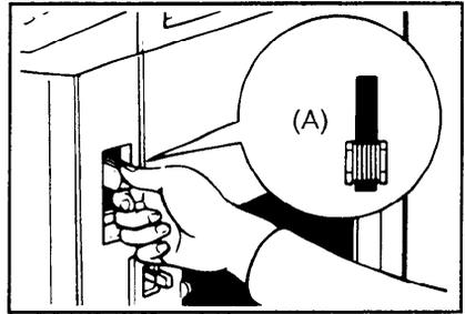
**2** Is the separation roller pressure properly adjusted?
