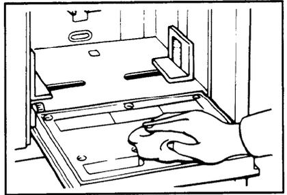
Make sure that the paper feed side plates contact the paper lightly.
