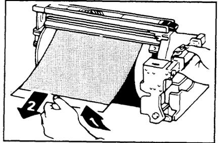
**4** Re-insert the drum unit until the drum unit locks in position and put the lever back in place.
