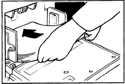
**5** Make sure that the paper feed side plates contact the paper lightly.
