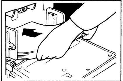
**4** Adjust the side plates and the end plate and if necessary, the small size end plate at paper delivery table.
