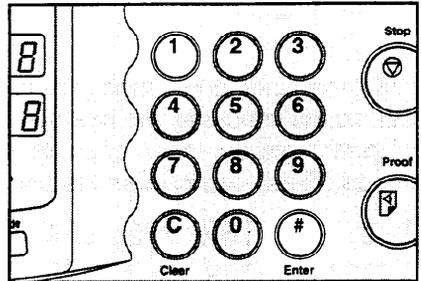
**4** Specify the Auto Reset time. Enter the desired setting using the **Number** keys and press the **Enter** key.
