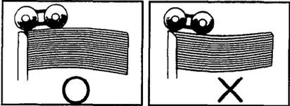
When the leading edge margin of the original is less than 5 mm, 0.2" or there is a solid image on the leading edge, insert the original with the widest margin first or make a leading edge margin by making a copy.
