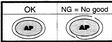
Draw the line at least 2 mm, 0.08", from the image so that the complete image can be recognized.
