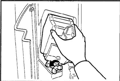
**3** While pushing the stopper down, push the knob to your side. Then, open the stapler unit cover.
