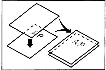
**2** Using a black, red, or blue felt tip pen, draw a line around the area to designate. The line should have a thickness of at least 2 mm, 0.08". Make sure there is no break in the line.
