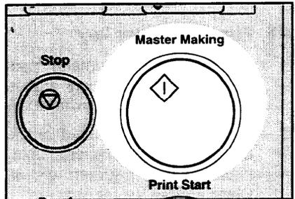
**8** The beeper sounds after the command sheet is scanned. Set the original face down on the exposure glass and press the **Master Making** key.
