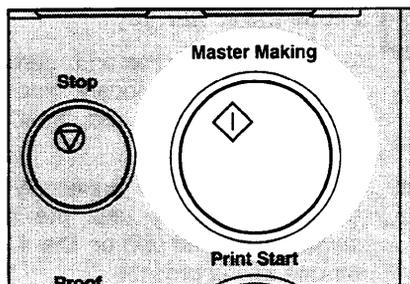
**10** The beeper sounds after the command sheet is scanned. Set the original face down on the exposure glass and press the **Master Making** key.
