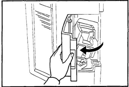
**2** Lift the empty staple cartridge a little and remove it from the stapler unit.
