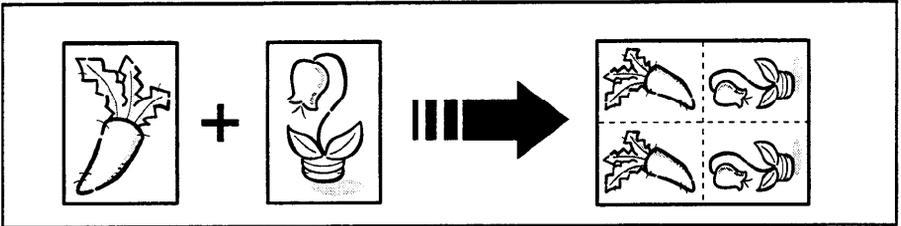
You can print 4 original images on a single sheet of paper using 2 originals. The images are positioned on the print as shown above. The following tables list the combinations that can be used when combining originals.
