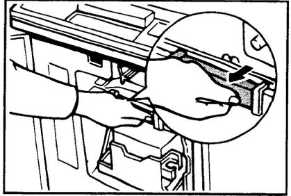
**5** Hold the rail on the drum and slide out the drum while pulling the release towards you.
