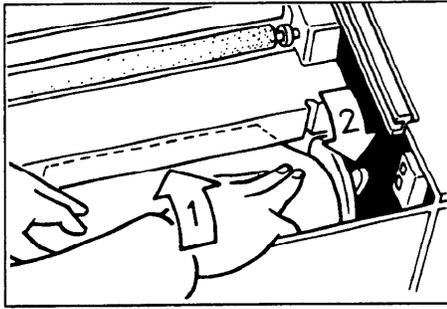
5. Insert the master from its roll under the arrow mark (1) until the leading edge comes out the other side of the steel cover.
