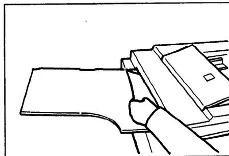
3. If you cannot remove the misfed original, pull out the original from the side of original delivery or open the original table and remove the original.
