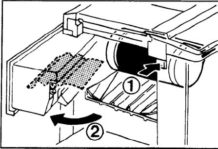
1. Press the master eject unit open button and open the master eject unit.
