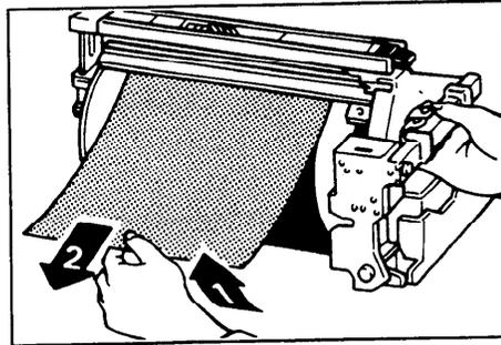
3. Remove the paper that is stuck to the drum.
