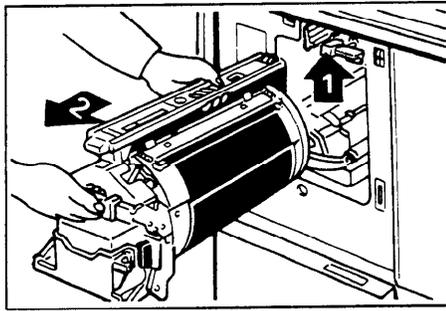
1. Lift the lever to unlock the drum unit and pull out the unit.
