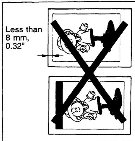
When the leading edge margin of the original is less than 8 mm, 0.32" or there is a solid image on the leading edge, insert the original with the widest margin first or make a leading edge margin by making a copy.
