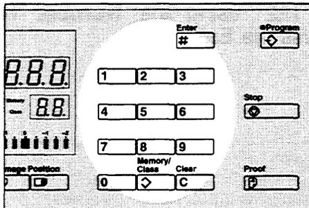
2. Enter "123" using the **Number** keys and press the **Enter** key.
