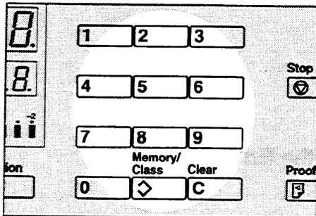
7. Using the **Number** keys, select the Image Make-up mode to be applied to the next command sheet. (See page 5.)
