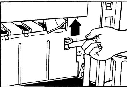
7. If printing on A3, 11" x 17", or larger paper, push up the wing guide release lever. If you want to print on paper smaller than A3 or 11" x 17", push down the release lever.
