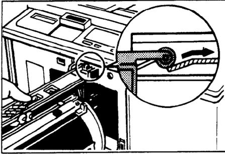
7. Insert the color drum unit along the guide rail.
