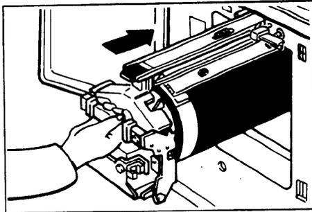
4. Insert the drum unit until it locks in position, then lower the drum unit lock lever.
