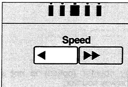
2. Reduce the printing speed by pressing the "◀" key.
