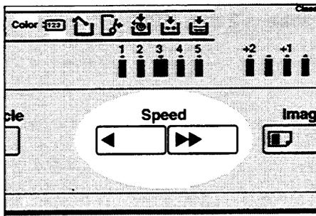
Press the **Speed** keys. To increase the speed, press the "▶" key. To reduce the speed, press the "◀" key.
