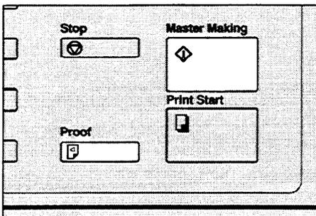
7. Press the **Master Making** key. Check the image position by making prints with the **Proof** key.
