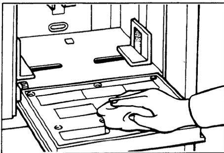
Wipe off the paper dust on the paper size detection sensors with a dry cloth.
