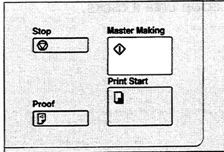
Set the original on the exposure glass and press the **Master Making** key.
