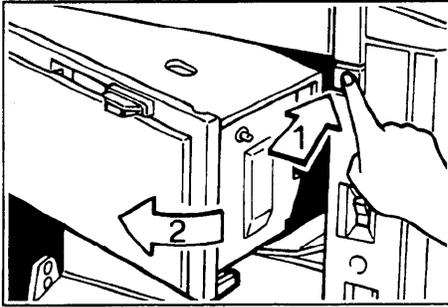
1. Push the button to open the master eject unit.
