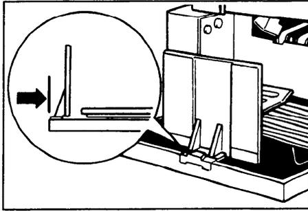
6. Move the end plate until the plate handle is flush with the end of the table.
