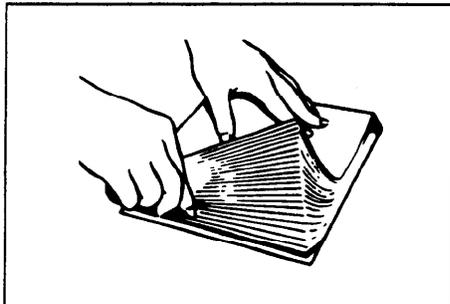
When paper edges stick together, shuffle the paper as shown.
