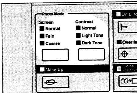
3. Adjust the screen image by pressing the **Screen** key, if necessary.
