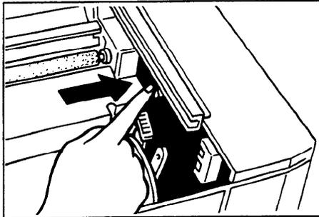
6. Return the pressure release lever to its original position.(2)
