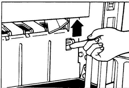
4. Set the wing guide release lever to match the print paper size.
