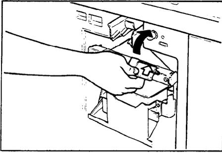
3. Lift the lock lever until it locks in position.
