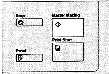
3. Press the **Master Making** key. Check the image position on the trial prints. (See page 16.)
