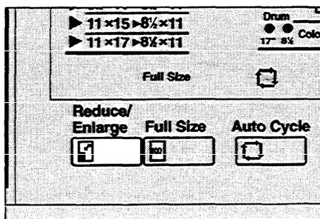
1. Select the desired enlargement ratio using the **Reduce/Enlarge** key.
