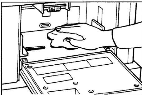
Wipe off the paper dust on the paper end sensor with a dry cloth.
