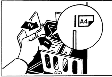
9. If you want to use paper A4, 8 1/2" x 11" or smaller, lift the small size paper delivery end plate and move it to match the print paper size.
