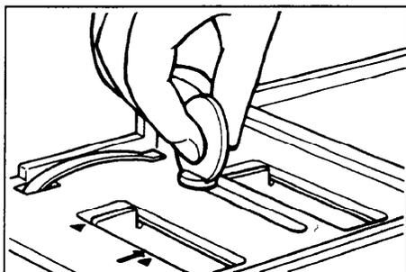
3. Loosen the 6 screws fixing the guide plate at the right, left, and rear sides.
