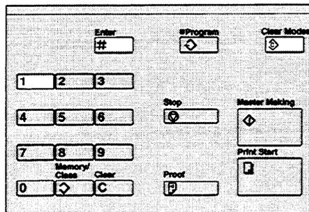
4. Enter "1" using the **Number** keys and press the **Enter** key.
