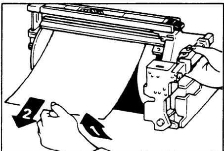
4. If you cannot remove the misfed paper, pull out the drum unit after confirming the lamp is green, and remove the misfed paper from the drum.
