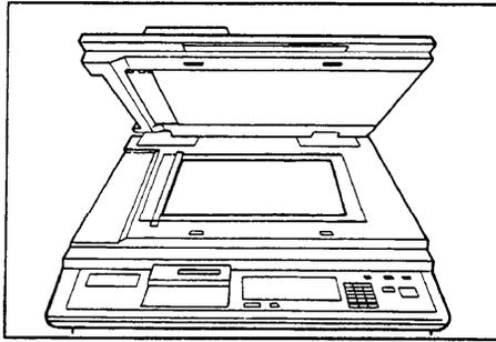
6. The beeper sounds after the first original is on the master. Set the second original face down and with the top toward the operating side.
