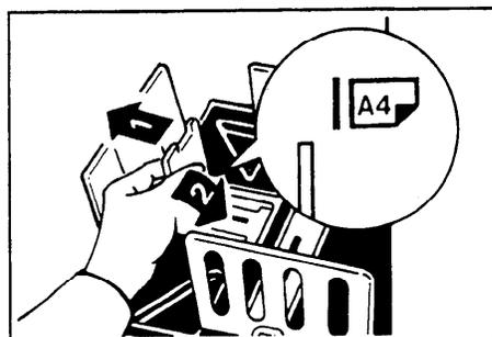
4. Push the small size paper delivery plate to the left, then lower it, if necessary.
