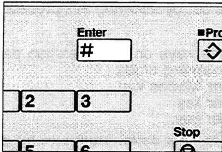
1. After entering the desired service program number, press the **Enter** key. The value or mode set at the factory will be displayed at the end of the second line on the guidance display.
