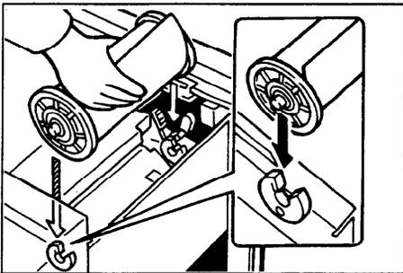
4. The new master roll must be positioned as shown in the illustration.
