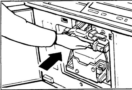
8. Slide in the drum unit until the drum unit locks in position.
