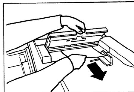
4. If the original misfeeds in the optional document feeder, press the ADF open lever and open the ADF unit to remove the misfed sheet.
