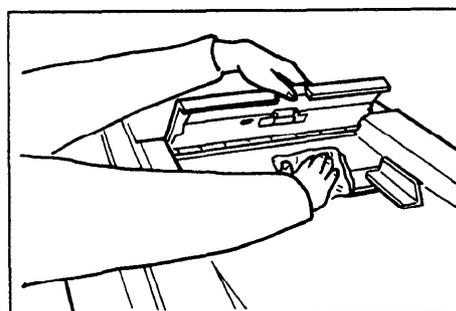
Clean the separation roller with a damp cloth and wipe it with a dry cloth.
