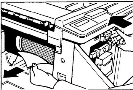
3. If the paper is completely wrapped around the drum, peel off the edge of the paper. Then, close the master eject unit and press the drum until the lamp turns green again. And then, open the master eject unit and remove the misfed paper.
