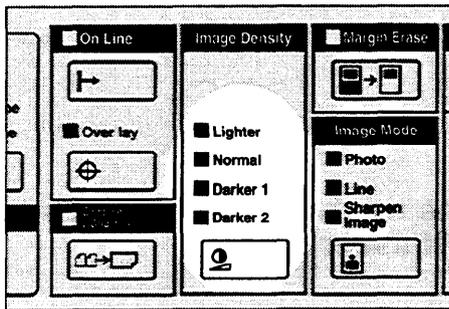
2. Press the **Image Density** key to adjust the image density.
