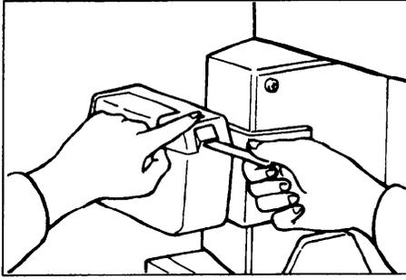
5. Press the manual cut button to trim off the leading edge of the tape.
