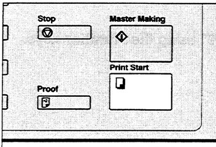
8. Check the image position of trial prints and press the **Print Start** key.
