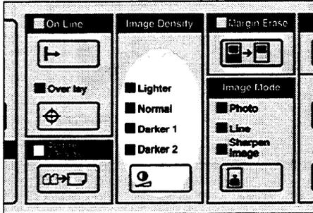
Use the **Image Density** key before pressing the **Master Making** key.
