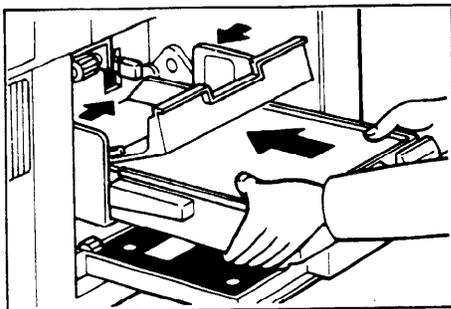
8. Push the cassette forward until it stops. Re-adjust the guide plates to the cassette size.
