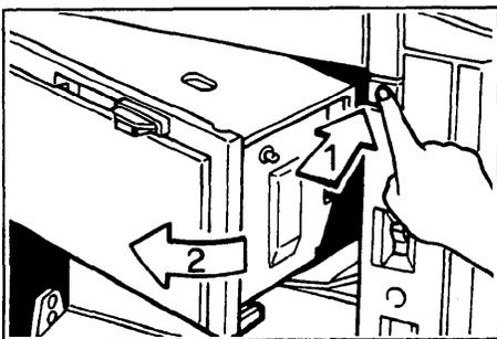
1. Push the master eject unit open button and open the master eject unit.
