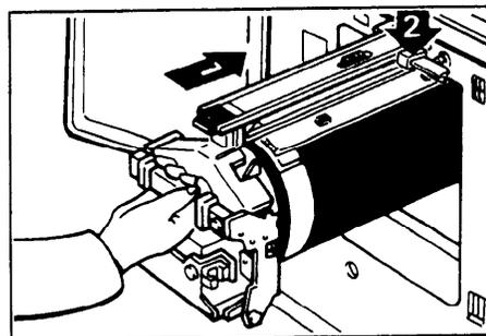
4. Reinsert the drum and put the lever back in place.
