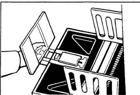
2. Is the paper delivery end plate in the correct position?
