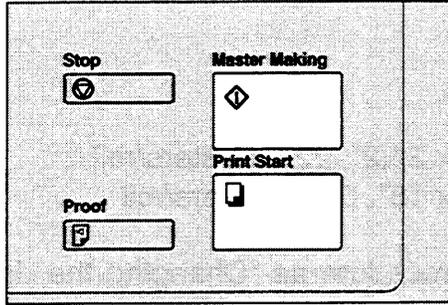
7. Set the second original and press the **Master Making** key. Check the image position. (See page 16.)
