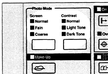
If you entered Fn4, adjust the screen and contrast with the **Screen** and **Contrast** keys.
