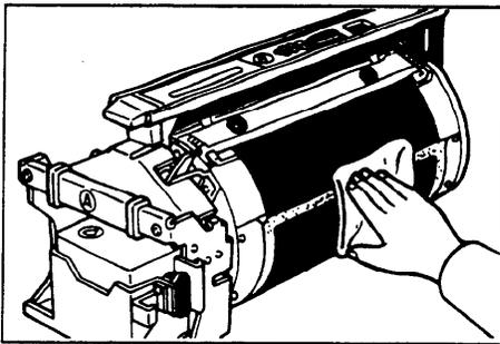
4. Remove with a clean cloth any ink that has accumulated on the trailing edge of the drum unit.
