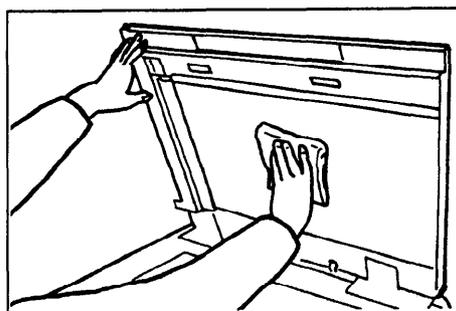
Clean the platen cover with a damp cloth and wipe it with a dry cloth.
