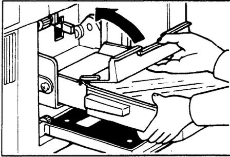
1. Press the **Paper Feed Table Down** key. Pull out the cassette to the middle of the paper feed table and close the cassette cover.
