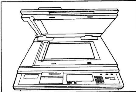
2. Place the original face down on the exposure glass. The original should be centered according to the size marks on the left scale.
