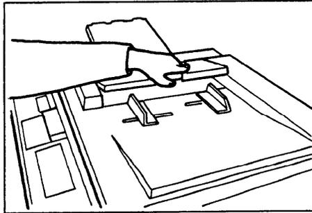
1. Press the ADF unit open lever and open the ADF unit.
