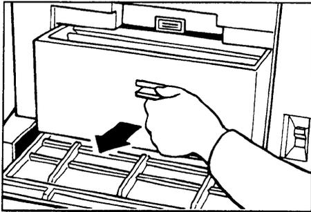
1. Open the master eject container cover. Then, pull out the master eject box.
