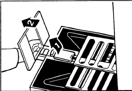
6. Lift the paper delivery end plate and move it to match the print paper size.
