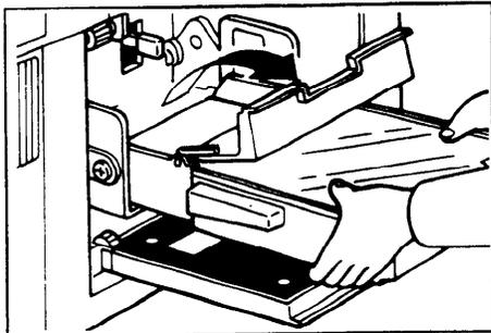
7. Using both hands, insert the cassette in the machine and open the front section of the cover, as shown.
