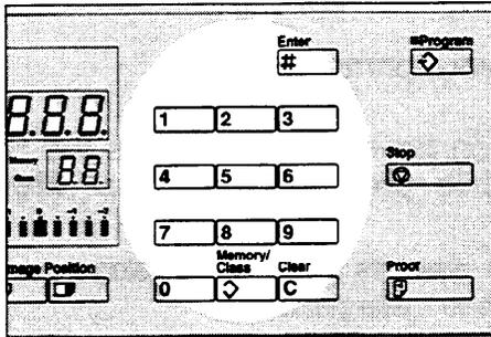
2. Enter "121" using the **Number** keys and press the **Enter** key.
