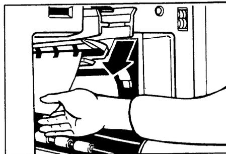
3. If you could not remove the misfed master in step 2, take out the drum and remove the misfed master from inside. (For how to take out the drum unit, see page 55.)
