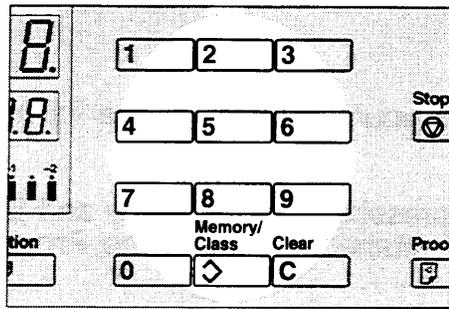
5. Enter one of the program numbers displayed on the guidance display using the **Number** keys.
