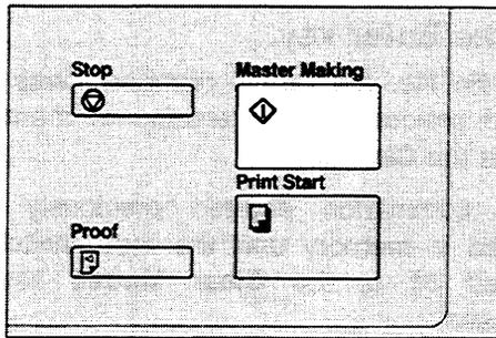
8. Set the command sheet face down on the exposure glass and press the **Master Making** key.
