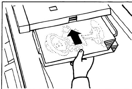
1. Insert the 2 originals face down and with the top toward the operation side.
