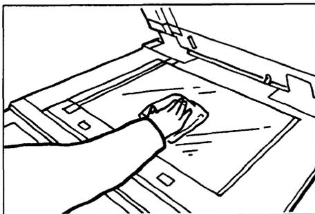
Clean the exposure glass with a damp cloth and wipe it with a dry cloth.
