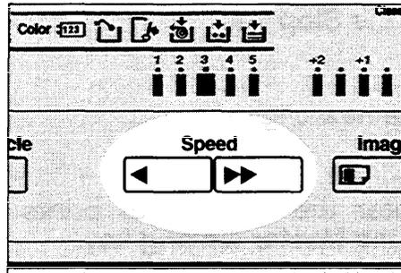
Press the **Speed** keys. To increase the speed, press the "▶" key. To reduce the speed, press the "◀" key. The printing speed will be changed as follows:
