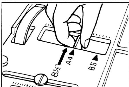
4. Slide the guide plates to the desired position and tighten the screws.
