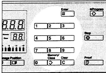
1. Input your assigned 3-digit user code using the **Number** keys, then press the **Enter** key.
