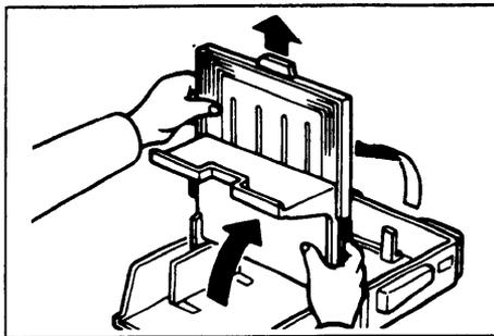
1. To remove the cassette cover, raise both sections of the cover to the vertical position, then pull the cover up and out from its holders.
