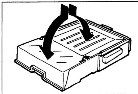
3. To replace the cover, fold both cover sections together and insert the cover as shown into the holders on the sides of the cassette.
