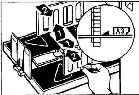
8. Lift the paper delivery side plates and adjust them to the paper size.
