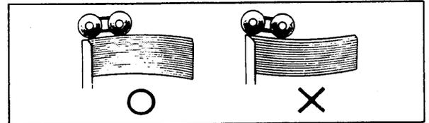
4. Make sure that the paper feed side plates contact the paper lightly.
