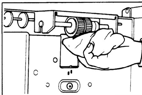
Wipe off the paper dust on the paper feed roller with a damp cloth, then wipe it with a dry cloth.
