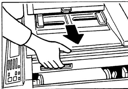
8. After the beeper sounds, remove the cut-off portion of the master roll.
