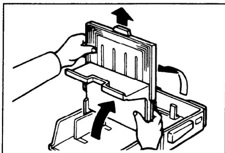
1. To remove the cassette cover, lift both sections to the vertical position and pull the cover up and out from its holders.
