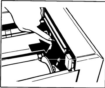
7. Press the master cut button to cut the leading edge of the master roll.
