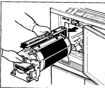
5. Remove the drum unit from the machine while holding the upper drum stay.
