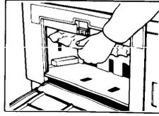
2. Remove the misfed master from master eject section.
