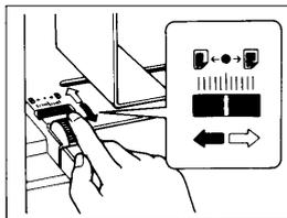
Turn the side plate fine adjusting dial. You can shift the image position to the right or the left up to 10mm/0.40" from the center.
