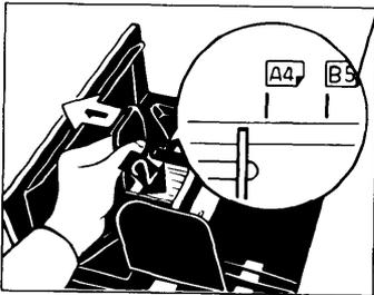
3. Return the small size paper delivery end plate to its original position.
