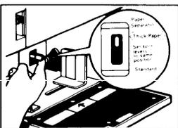
4. If the separation roller pressure lever is in the standard position, move it to the thick paper position.
