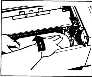
5. Insert the leading edge of the master roll under the pressure roller.(1)
