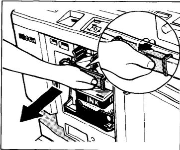
3. Pull out the drum unit handle while pressing the release bar inside the green handle.
