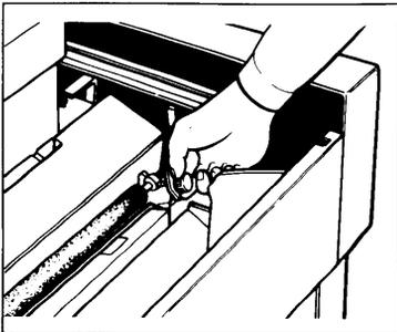
4. Loosen the screw knobs located on both sides of the feed roller.
