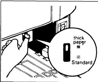
1. Push down the feed roller pressure lever.
