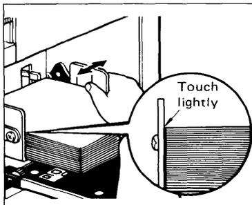
4. Adjust the paper delivery side plates and the paper delivery end plates.
