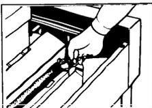
Check that the installation screws on both sides of the master feed roller are secured.
