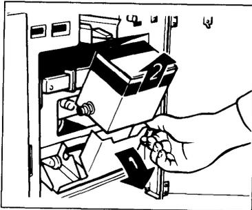
2. Lower the ink holder and remove the used ink cartridge.
