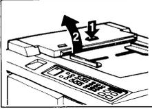
1. Press the ADF unit open button and open the ADF unit.
