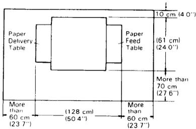
Place the machine near a power source, providing clearance as shown to the left.
