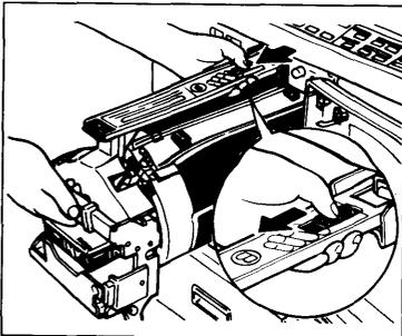
4. Hold the rail on the drum and slide out the drum while pressing the release slide to the front.
