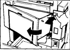
1. Push the master eject unit open button and open the master eject unit.
