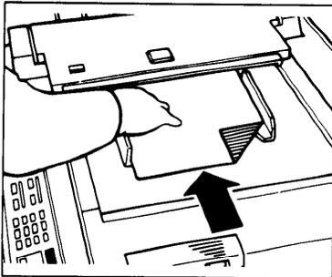
2. Insert the original face down on the original table until it stops.
