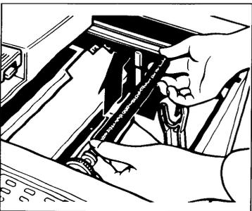
5. Grip both ends of the feed roller and lift it straight up.
