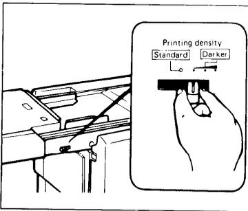
2. Adjust the printing density to match the type and quality of the original using the printing density select switch.
