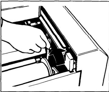
2. Lift the pressure release lever in the direction of the arrow to release the feed roller pressure.
