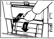
1. Open the master eject container cover and remove the master eject box.
