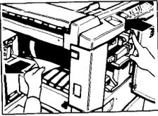
3. When paper is wrapped around the drum, open the front cover and remove the paper while rotating the drum by pressing the drum rotation button.
