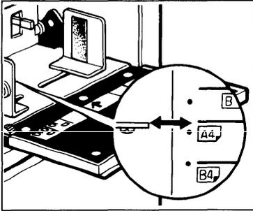
2. Adjust the paper feed side plates to match the paper size.
