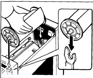
4. The new master roll must be positioned as shown in the illustration.
