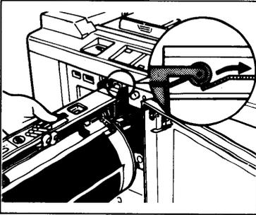
6. Insert the color drum unit along the guide rail.
