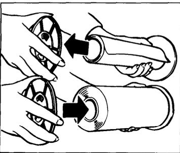
3. Remove the used master roll and pull out both spools. Then, insert both spools into a new master roll.
