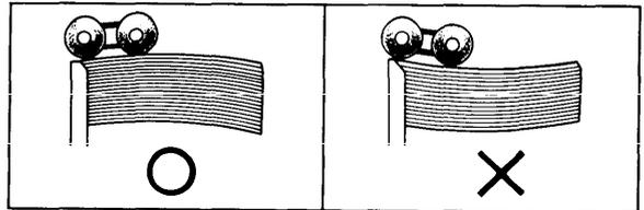
4. Make sure that the paper feed side plates contact the paper lightly.
