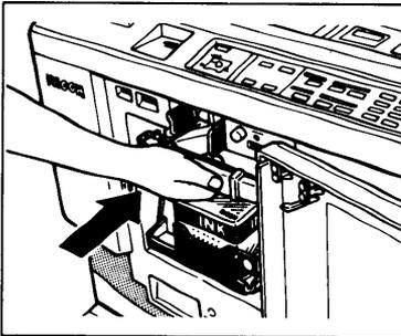
7. Slide in the drum unit until the drum unit locks securely.
