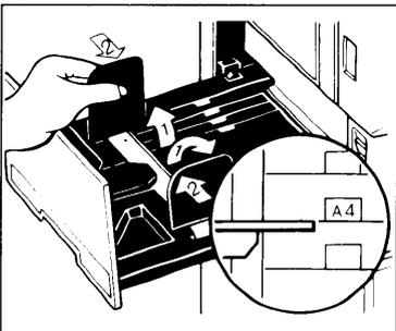
6. Lift the paper delivery side plates and adjust them to the paper size.
