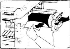
When paper is completely wrapped around the drum, pull out the drum unit until the drum hits the drum stopper, and remove the misfed paper from the drum.
