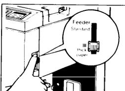
2. If the feed roller pressure lever is in the standard position, set it in the thick paper position.
