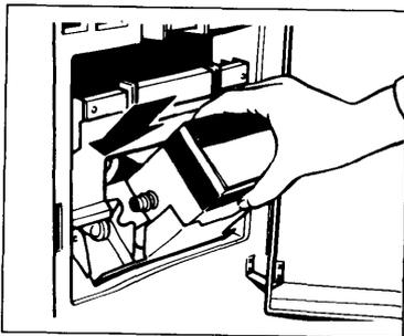
3. Remove the cap of the new ink cartridge and insert the new cartridge into the ink holder. Return the ink holder to its original position.
