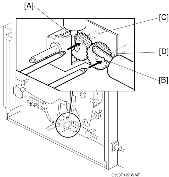
**Purpose:** To ensure that the paper pawl air pump produces a jet of air when the paper exit pawl is in the upper position (near the drum surface)
