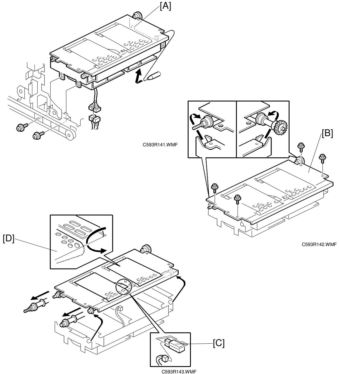
1. Remove the relay transport delivery table unit [A] (2 screws, 2 connectors).
