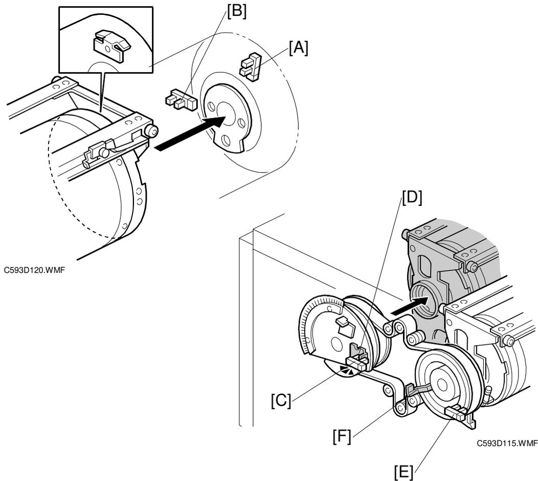
The 1st jam sensor [A] and the 2nd jam sensor [B] generate timing signals for paper jam detection. These sensors are at the rear of the 1st drum.
