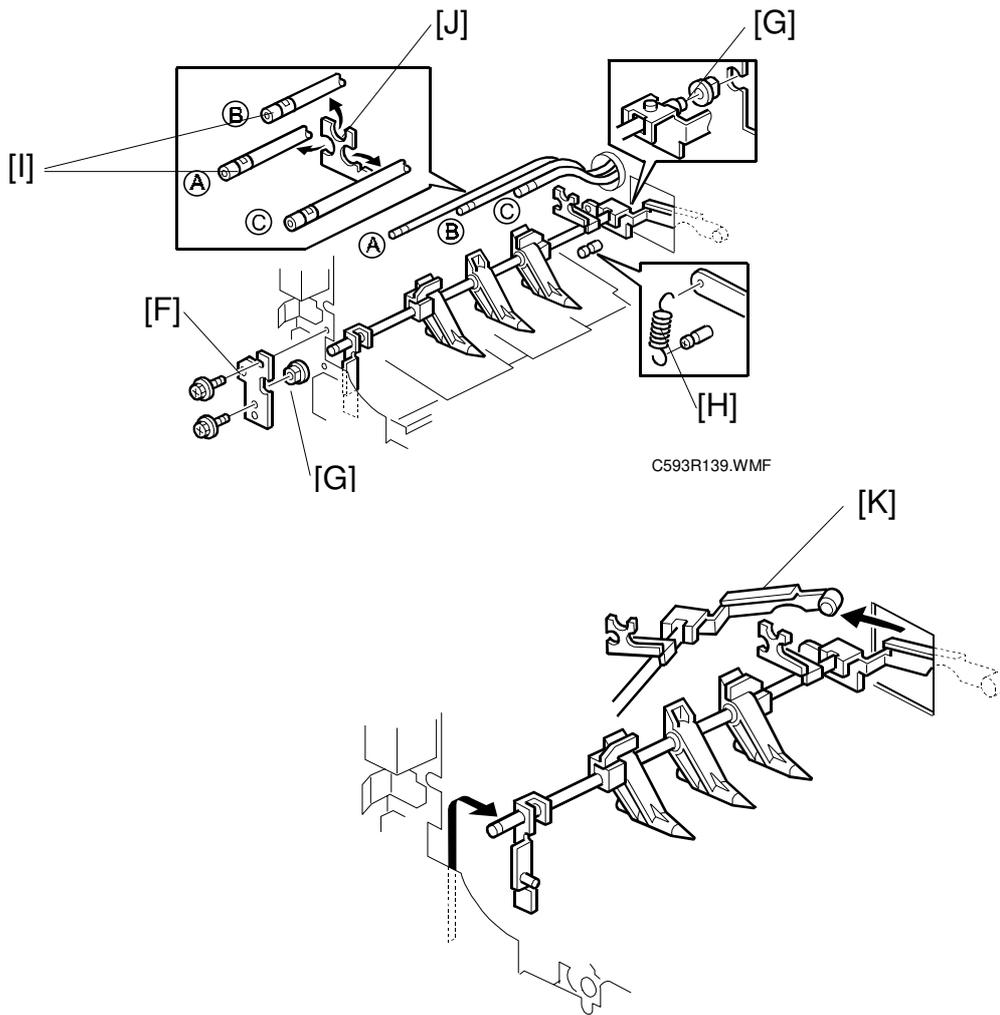
7. Remove the exit pawl shaft bracket [F] (2 screws).
