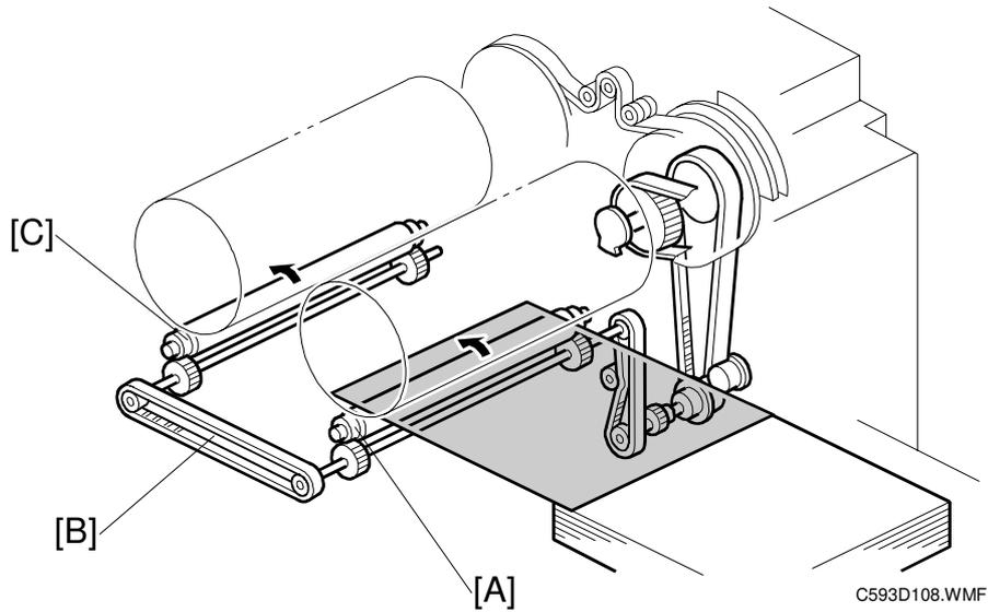
The main motor (not shown) drives the press roller [A] for the 1st drum through timing belts and gears.
