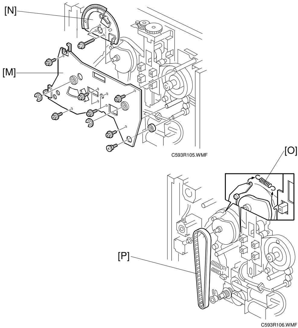
15. Remove the side plate [M] (2 e-rings, 9 screws, 3 bearings).
