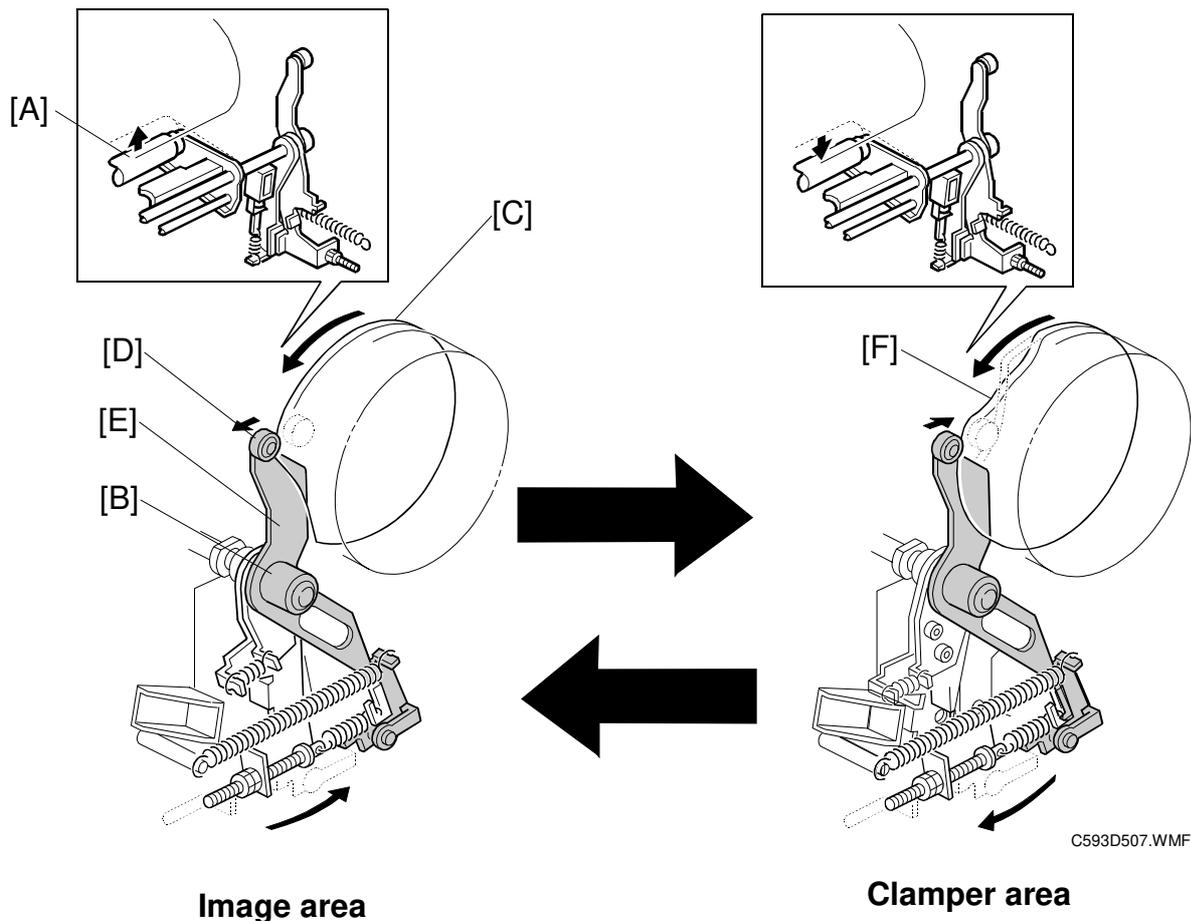
When the arm and the lever are interlocked, the press roller [A] is lifted when the arm shaft [B] turns.
