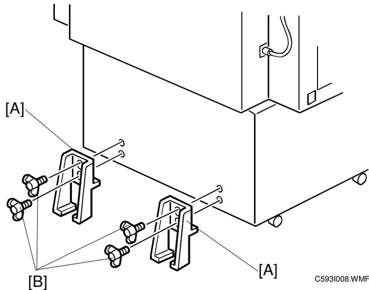
6. Attach the two stabilizer brackets [A] to the back of the table using the thumbscrews [B] (4 screws). All components are in the accessories.
