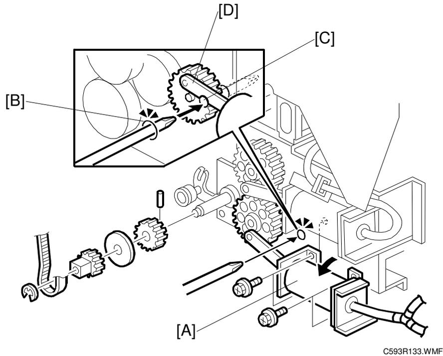
1. Remove the lower air pump [A] (4 screws).
