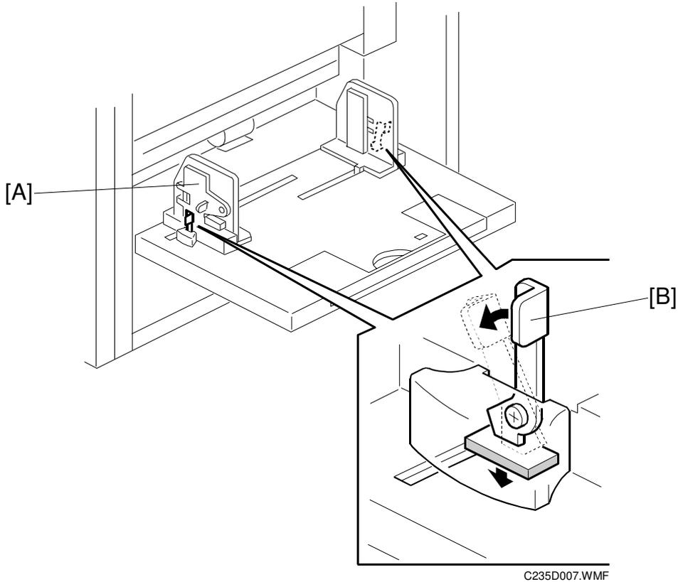
The left and right side fences [A] move together due to a rack and pinion mechanism. There is a lock lever [B] to hold the side fences in position.
