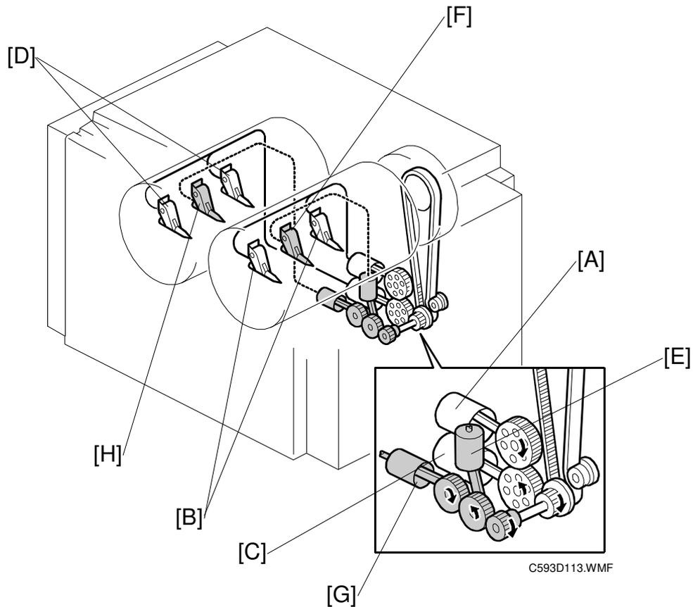
The main motor drives the air pump pistons through gears. The pistons push a jet of air out through the nozzles in the exit pawls. The jets of air push down on the paper and separate it from the drum.
