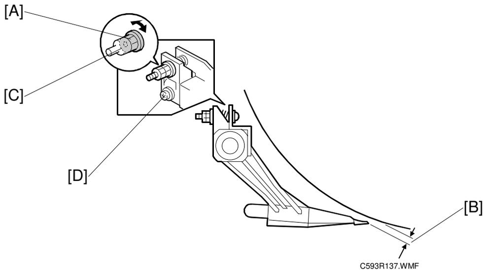
1. If adjusting the gap for the 1st drum, move the 2nd drum to its removal position. Do the opposite when adjusting the gap for the 2nd drum.
