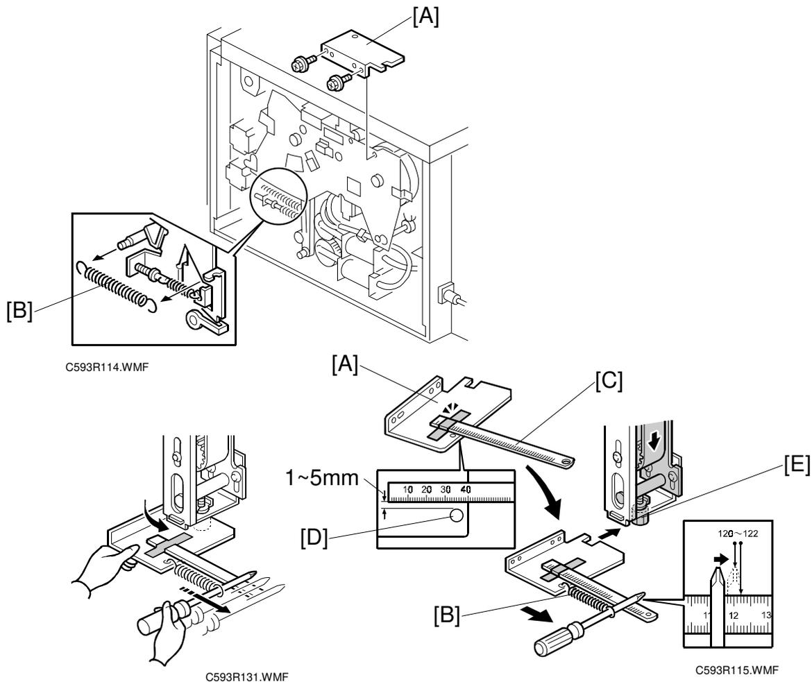
1. Remove the 2nd drum safety cover [A] (2 screws).
