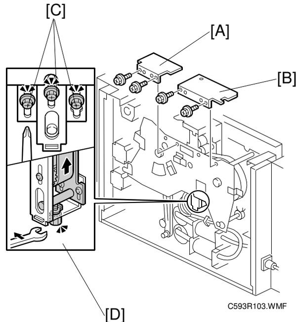
1. Turn on the main switch and access SP601 (registration adjustment) and SP602 (drum synchronization adjustment).
