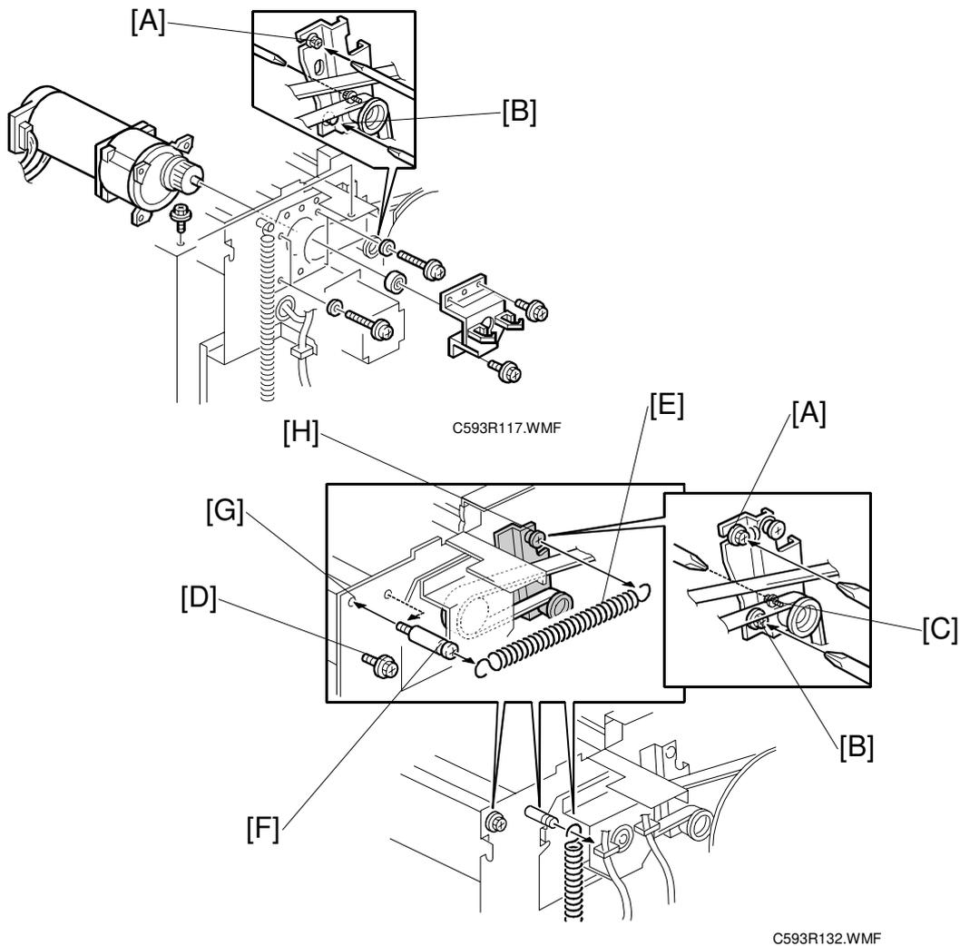
1. Loosen screws [A], [B], and [C] to about half way.
