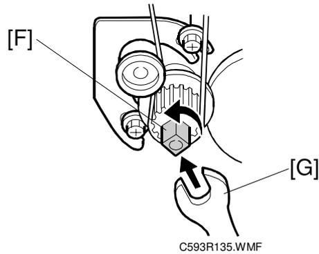
7. Rotate the pump drive shaft [F] with a wrench [G] until the drum holding unit completes 1 rotation.
