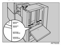
**2** Tighten the screw to lock the side guides.
