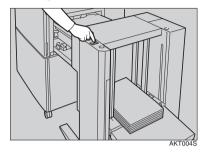
At the machine, adjust the side guides of the paper feed tray to the paper size set for the LCIT and check that the paper size is displayed on the control panel.
