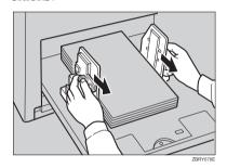
To print on thin paper (52.3g/m<sup>2</sup>, 13.9 lb), slide the levers behind the paper feed side plates in the direction of the arrow (see illustration).
