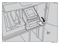
Insert the drum unit along the guide rail.
