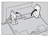
Make sure that the locklever for the side plate is raised (lock is released), and then grasp the side plate knob and adjust the side plate to match the paper size.
