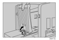
2 Adjust the angle of the end plate by turning the screw clockwise or counterclockwise.
