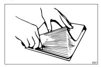
• When printing onto envelopes or thick paper, lower the printing speed. ⇒ p.32 "Changing the Printing Speed".
