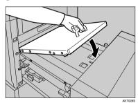
② Move the cover release lever back to the original position.
