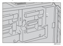
4 Lower the drum unit lock lever B1.
