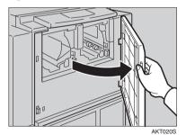
Lift upper drum stay B3 a little to unlock the drum unit, then push into the drum unit while holding drum unit handle B2 and upper drum stay B3.
