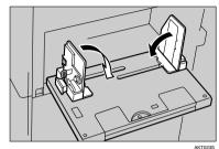
Hold the handle and unfold the intermediate feeding section of the LCIT.
