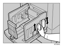
Adjust the paper alignment wings and chocks according to paper size and thickness, as follows: When printing on thick paper (128 g/m<sup>2</sup>, 34 lb or thicker)
