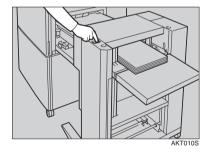
The input tray goes up and a sheet of paper is fed into the intermediate feeding section. The green indicator stops blinking and stays lit.
