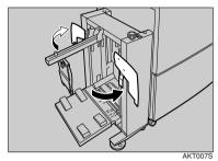
2 Loosen the screw for the end plate, move it as close to the machine as possible, and then tighten the screw to lock the end plate.
