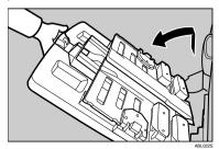
2 Lift the paper delivery side plates and adjust them to match the paper size.
