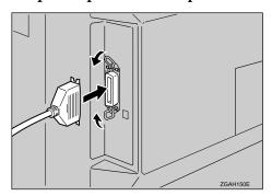
Plug the other end of the parallel cable into the computer's parallel port.
