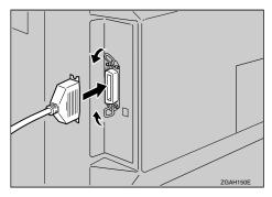
3 Plug the other end of the parallel cable into the computer's parallel port.
