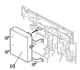
**NOTE:** After installing the printer controller unit, make sure that the board and the cable are securely connected.
