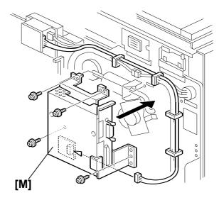
**NOTE:** After installing the printer controller unit, make sure that the board and the cable are securely connected.
