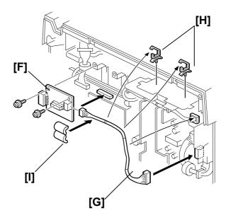
NOTE: 1) Install two cable clamps [H]. Then clamp the power cable.
