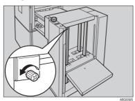
Turn the side guide adjustment knob to adjust the side guides to the new paper size.
