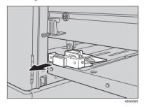
While pulling the LCIT release lever, detach the LCIT.
