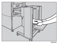
Remove the paper remaining in the intermediate feeding section.
