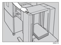
The input tray goes up, and a sheet of paper is fed into the intermediate feeding section. The green indicator lights.
