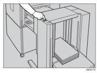
5 At the machine, adjust the side guides of the paper feed tray to the paper size set for the LCIT and check that the paper size is displayed on the control panel.
