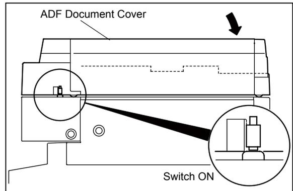
When the ADF document cover is open, the actuator is released; the micro switch is turned to CLOSE.
