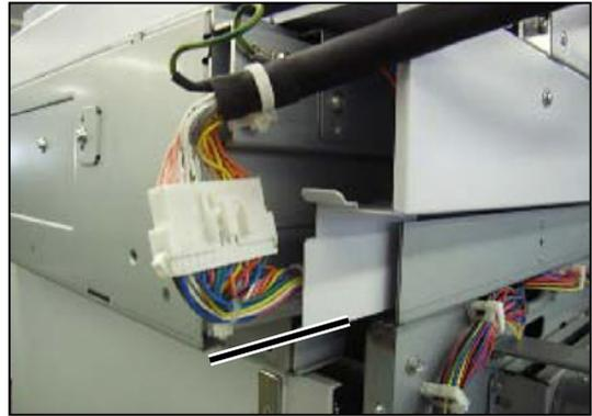
5. Remove the two screws, and slide the ADF document cover 1 cm and pull it out upward.
