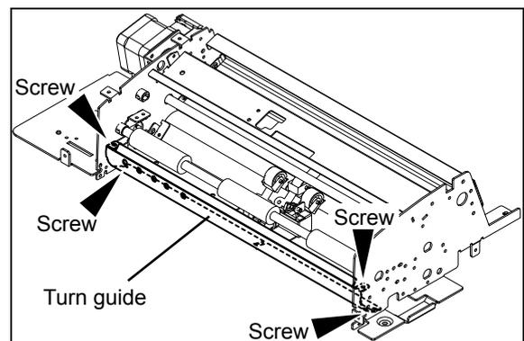
4. Remove the screw, together with the bracket.
