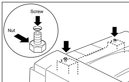
**(3) Removing the ADF Front / Rear Cover**
