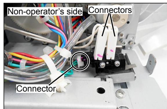
4. Remove the two screws to remove the ADF document cover open/close switch and ADF document cover open/close switch 2.
