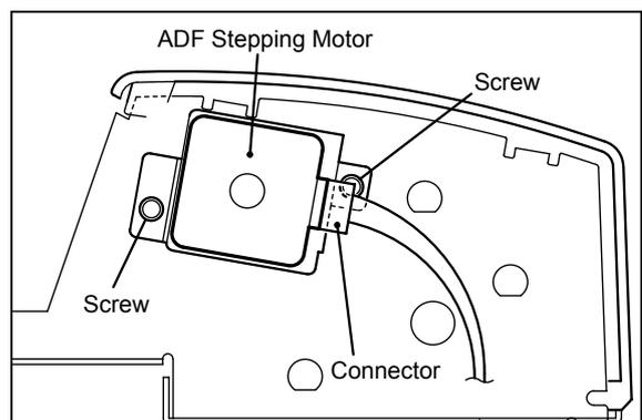
5. Remove the two screws to remove the motor bracket.
