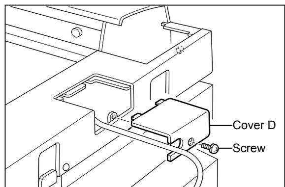
4. Disconnect the two connectors and remove one screw.
