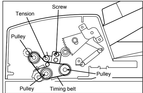
**3****(8) Removing the ADF Clutch A/B**
