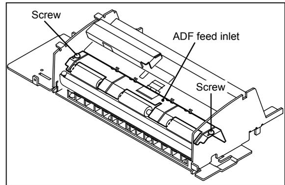
3. Remove the four screws to remove the turn guide.
