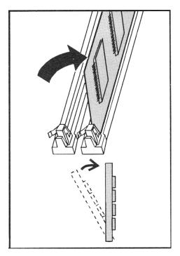
Figure B-1.10. Securing the SIMM board in the socket.
