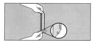
Figure B-1.8. Positioning the SIMM.
