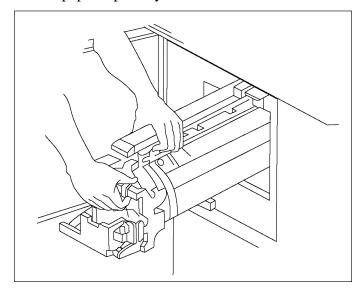
Figure 1-1.9. Load the color drum into the digital duplicator.
