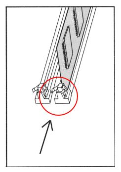
Figure B-1.6. Locate the SIMM locking tabs.
