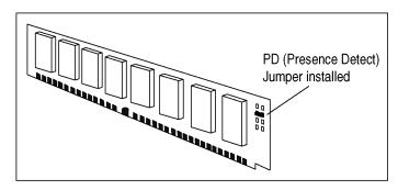
Figure B-1.1. Example of a single-sided SIMM with one PD jumper installed.
