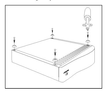
Figure B-1.3. Removing top cover hold-down screws.
