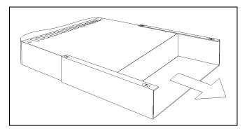
Figure B-1.4. Removing top cover.
