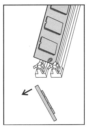
Figure B-1.7. Removing an existing SIMM board.
