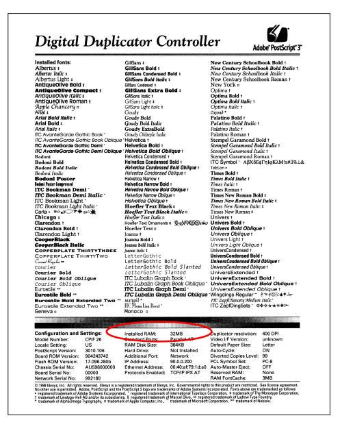
Figure B-1.12. Using the Diagnostic Test Page to verify correct memory installation.
