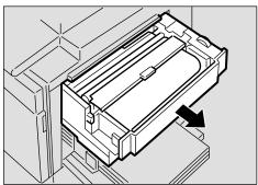
2 Open the black cover at the bottom of the master tray and remove turn scraps of the master.
