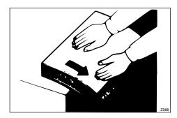
When the leading edge margin of the original is less than 8mm, 0.32" or there is a solid image on the leading edge, insert the original with the widest margin first or make a leading edge margin by making a copy.
