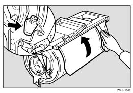
With a dry soft cloth, remove any ink that has accumulated on the trailing edge of the drum unit.
