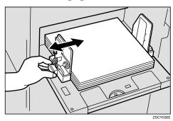
Push the lock lever for the paper feed side plates down to lock the side plates into position.
