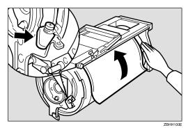
6 Insert the drum unit until it locks in position, and then lower the drum unit lock lever.
