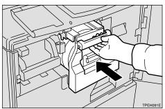
**9** Lift drum unit lock lever B1.
