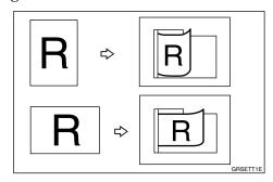
If the original is place in a different direction from the print paper, the machine automatically rotates the original image by 90° to match the print paper direction.
