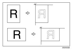
When the original is placed in a direction that differs from the print paper, the machine automatically rotates the original image by 90° to match the print paper direction.
