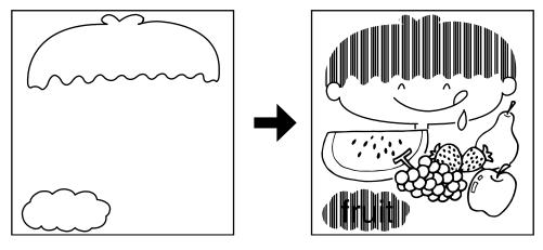
The closed line method is easier to use for complex areas, but it is less precise. It also takes longer to draw a command sheet with the closed line method.
