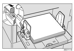
Re-adjust the paper feed side plates so that there is no space between the paper feed side plates and paper, and then lock the side plates in position.
