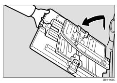
Raise each paper delivery side plate, and then grasp the side plate knobs and move the paper delivery side plates to match the print paper size.
