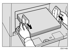
To print on thin paper (47.1g/m², 12.5 lb), slide the levers behind the paper feed side plates in the direction of the arrow (see illustration).
