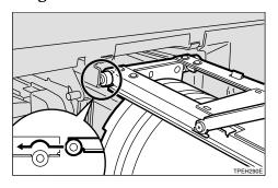
**1** Lower the drum unit lock lever (B1) of the inserted drum.
