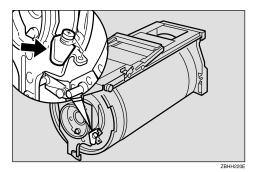
Insert the color drum unit along the guide rail.
