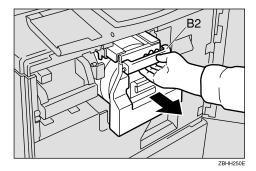
Lift the upper drum stay (B3) a little to unlock the drum unit, and then pull out the drum unit while holding the drum unit handle (B2) and the upper drum stay (B3).
