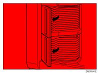
2 If the misfed paper is deep inside of the bin and you cannot remove it, press the green button 2 while pressing the button ①. When the misfed paper is pushed out, remove it from the sorter.
