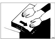
When paper edges stick together or paper is not fed in, shuffle the paper as shown.
