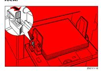
Re-adjust the paper feed side plates so that there is no space between the paper feed side plates and paper, and then lock the side plates in position.
