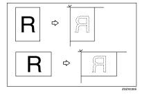
When the original is placed in a direction that differs from the print paper, the machine automatically rotates the original image by 90° to match the print paper direction.
