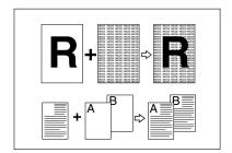
Combines the images of originals stored in Original Storage with the originals placed on the machine.
