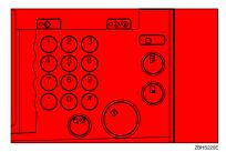
After the first set is completed, place the second original on the exposure glass, and then press the [Start] key.
