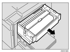
2 Open the cover at the bottom of the master tray while holding the lever and remove the fragments.
