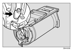
Insert the color drum unit along the guide rail.
