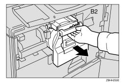
4 Lift the upper drum stay (B3) a little to unlock the drum unit, and then pull out the drum unit while holding the drum unit handle (B2) and the upper drum stay (B3).
