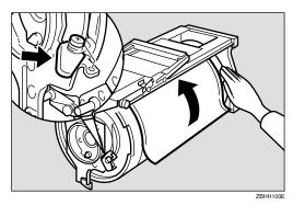
6 Insert the drum unit until it locks into position, and then lower the drum unit lock lever.
