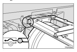
**7** Lower the drum unit lock lever (B1) of the inserted drum.
