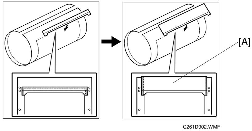
The adhesive parts [A] are only at the sides of the mylar seal for the metal screen. (They were removed from the trailing edge.) This prevents ink leakage from the trailing edge.
