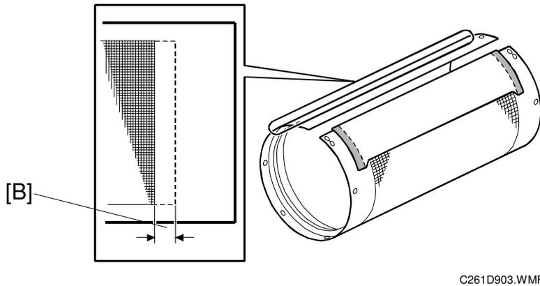
The leading edge of the mesh on the metal screen is reduced by 2.5 mm [B]. This prevents small dots at the leading edge of the paper.
