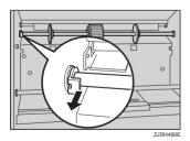
**4** Slide the shaft slightly to the left and lift it out from its right end.
