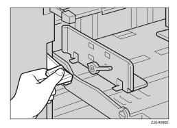
Release the paper feed side plate lock levers and adjust the side plates to match the paper size.
