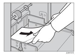
Release the paper feed side plate lock levers. Adjust the paper feed side plates to match the new paper size.
