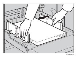
Shifting the image to the left Shift the paper towards the back of the machine.
