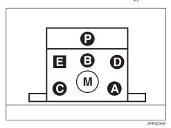
The machine indicator shows the place where the door/units are not closed.
