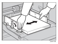
Shift the tray adjustment lever to the paper feeding position.
