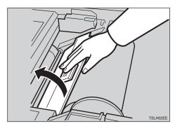
If you could not remove the misfed master in steps 2 and 5, take out the drum and remove the misfed master from the inside.
