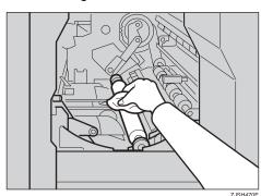
With a clean cloth, remove any ink that has accumulated on the trailing edge of the drum unit.
