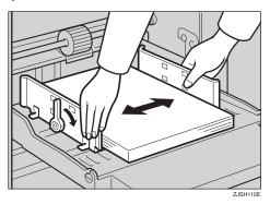
When you have finished printing, shift the feed roller pressure lever back to the Standard paper position.
