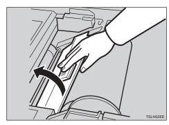
Remove the used master roll and pull out both spools. Then, insert both spools into a new master roll.
