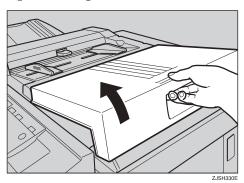
**2** Open the plotter cover, and then remove the misfed master.
