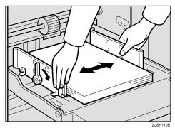
5 Shift the tray adjustment lever to the paper feeding position.
