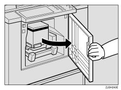
2 Release the ink holder lock lever and pull out the ink holder. Remove the used ink cartridge.
