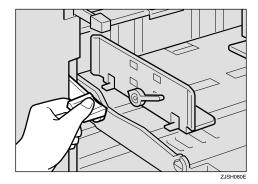
Release the paper feed side plate lock levers and adjust the side plates to match the paper size.
