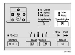
Press the [Image Density] key to adjust the image density.
