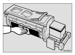
Insert the drum unit until it locks in position, then lower the drum unit lock lever.
