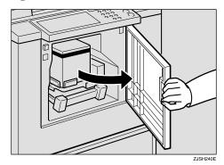
2 Lift the drum handle to unlock the drum.
