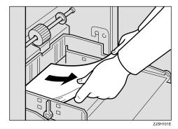
2 Release the paper feed side plate lock levers. Adjust the paper feed side plates to match the new paper size.
