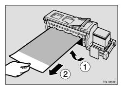
Remove paper that is stuck to the drum.
