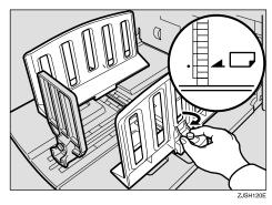
Adjust the paper delivery end plate to match the paper size.
